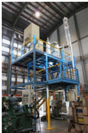
Plate 4.1. BCB Process – Binderless Coal Briquetting – pilot plant.
