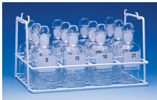
Figure 2.2 A rack of bottles used for measuring the Biochemical Oxygen Demand (BOD)
