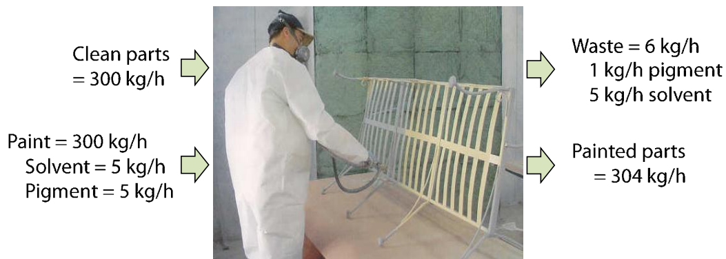
Figure 4.2 Paint spray booth material balance
