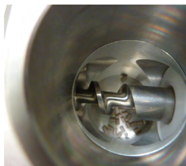
Figure 3.17 Hopper with an auger facility
