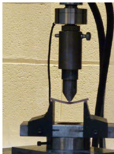
Figure 6.14 A specimen tested in 3-point bending
