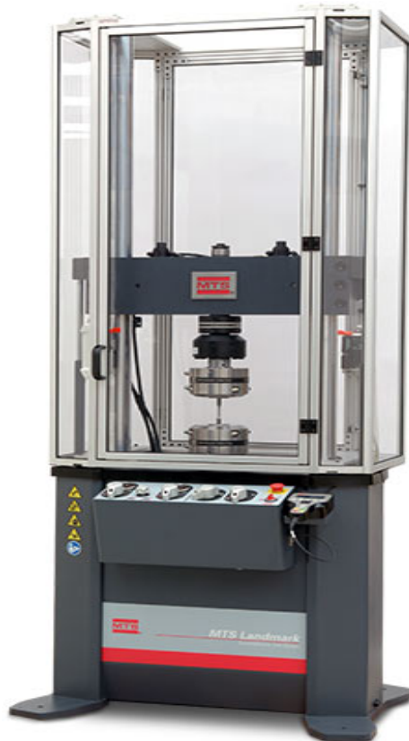
Fig. 2.6 MTS testing machine, see [ www.mts.com ]
