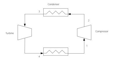
Figure 5.18: Air-standard refrigeration cycle.
