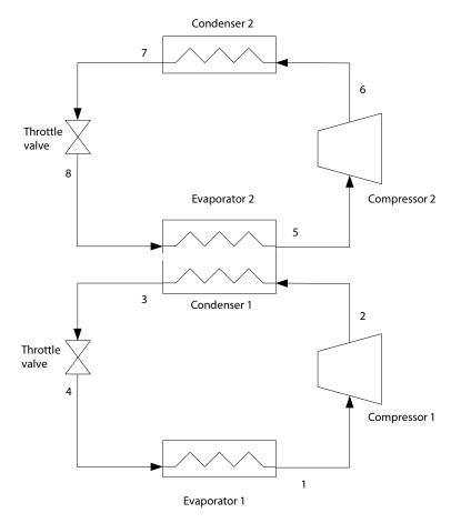
Figure 4.13: Vapour compression cycle using two evaporators.
