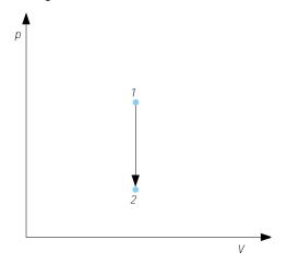
Figure 1.11: Constant volume process on a p-V diagram.
