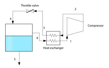
Figure 5.15: Linde-Hampson cycle components.
