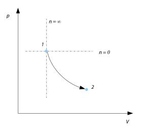
Figure 1.12: Polytropic process on a p-V diagram.
