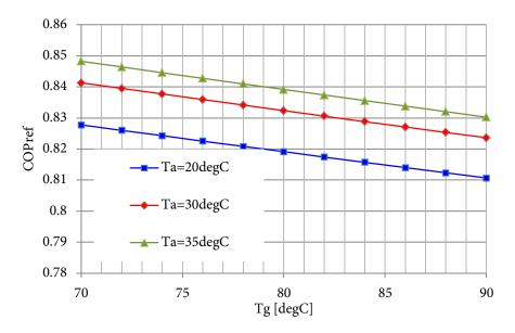
Figure 8.12: COP against generator temperature.
