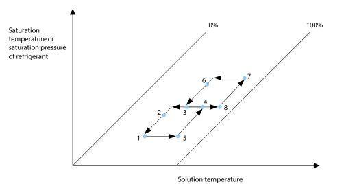
Figure 5.14: Dühring plot for a double effect vapour absorption system.
