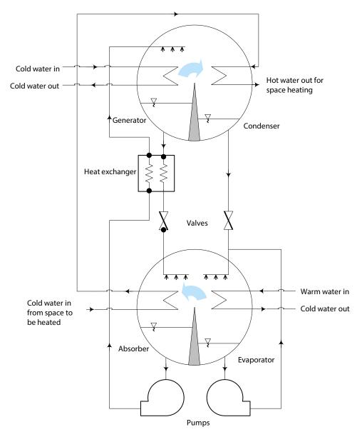
Figure 5.10: Single stage vapour absorption chiller/heat pump
