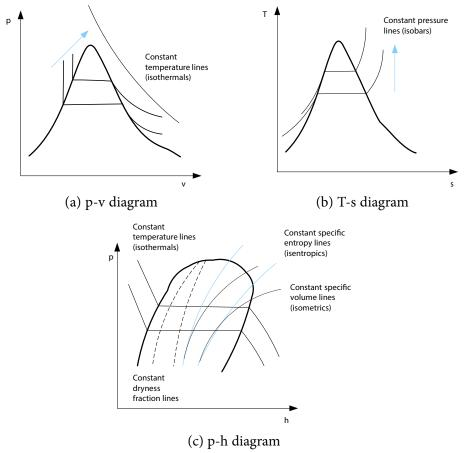
Figure 3.2: Important features of p-v, T-s and p-h diagrams. Arrows point towards increasing quantities.
