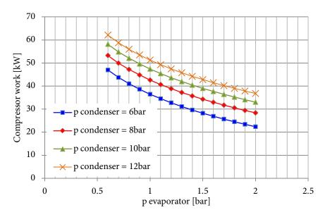
Figure 7.6: Compressor power against evaporator pressure for various condenser pressures.
