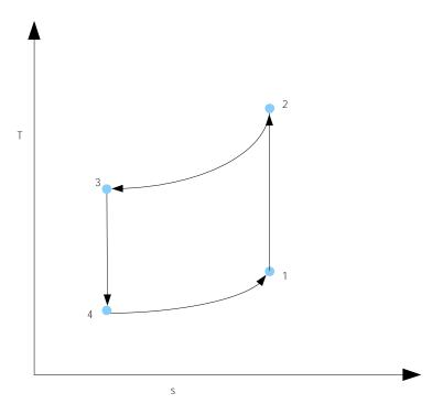
Figure 5.19: Air-standard refrigeration cycle T-s diagram.
