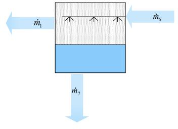
Figure 5.5: Generator mass transfer.
