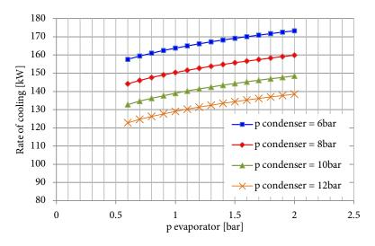
Figure 7.4: Rate of cooling against evaporator pressure for various condenser pressures.
