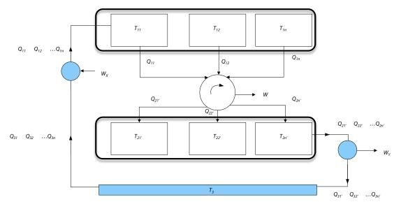
Figure 1.9: System operating between a finite number of reservoirs.
