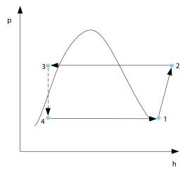
Figure 4.6: p-h diagram for a vapour compression cycle.
