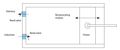
Figure 4.17: A reciprocating type compressor cylinder.
