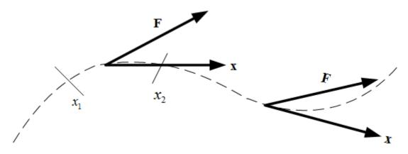
Figure 1.4: Concept of work done between two points.
