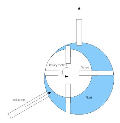
Figure 4.18: A rotary vane type compressor.
