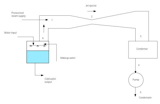
Figure 5.17: Steam jet refrigeration cycle.
