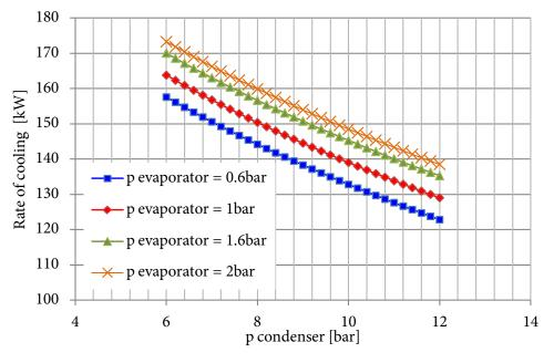
Figure 7.5: Rate of cooling against condenser pressure for various evaporator pressures.
