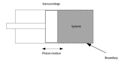
**Figure 1.2:** Piston work input on the system. System boundaries change dimension depending on the piston motion but no mass enters or leaves the system (closed system).
