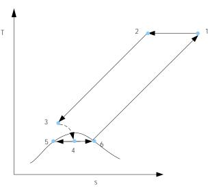
Figure 5.16: Linde-Hampson cycle T-s diagram.
