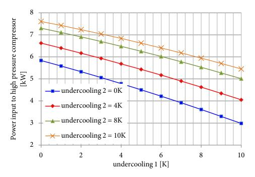
**Figure 7.12:** Power input to high pressure compressor against undercooling in the lower stage at various undercooling temperatures in the higher stage. The lower stage mass flow rate is set to 1kg/s while the higher stage compressor is set to 0.8kg/s.
