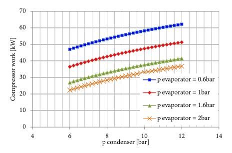
Figure 7.7: Compressor power against condenser pressure for various evaporator pressures.
