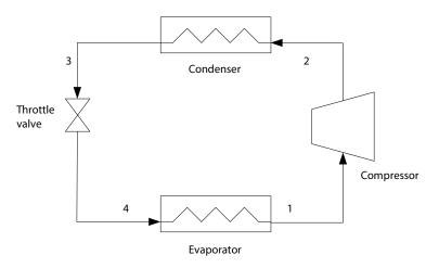
Figure 4.4: Components of a vapour compression cycle.
