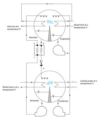
Figure 5.11: Single stage vapour absorption heat transformer
