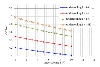
**Figure 7.15:** Refrigeration COP against undercooling in the higher stage at various undercooling temperatures in the lower stage. The lower stage mass flow rate is set to 1kg/s while the higher stage compressor is set to 0.8kg/s.
