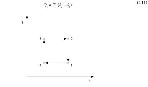
Figure 2.4: Carnot cycle T-S diagram for a reversed heat engine.
