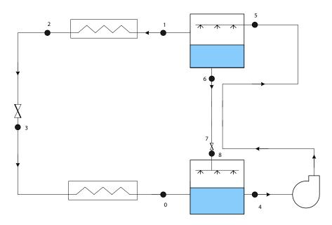
Figure 5.8: LiBr-water vapour absorption system without SHX.
