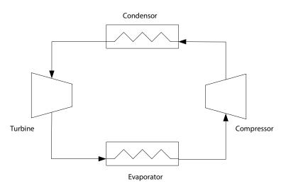
Figure 2.3: Reversed heat engine components.
