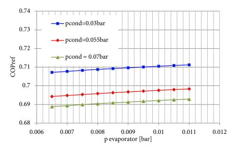
Figure 8.7: COP against evaporator pressure.
