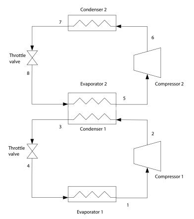
Figure 7.10: Model the cascaded system showing state points.
