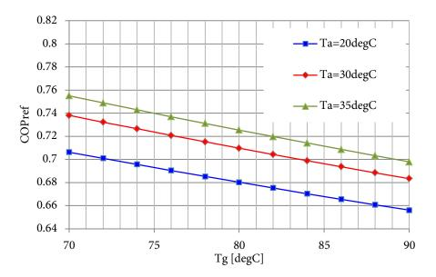
Figure 8.6: COP against generator temperature.
