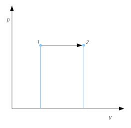
Figure 1.10: Isobaric process on a p-V diagram.
