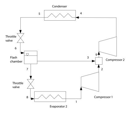
Figure 4.11: The multistage vapour compression cycle.
