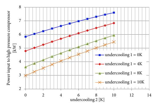
**Figure 7.13:** Power input to high pressure compressor against undercooling in the higher stage at various undercooling temperatures in the lower stage. The lower stage mass flow rate is set to 1kg/s while the higher stage compressor is set to 0.8kg/s.
