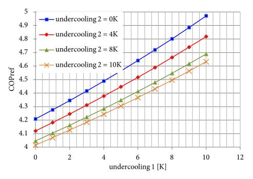
**Figure 7.14:** Refrigeration COP against undercooling in the lower stage at various undercooling temperatures in the higher stage. The lower stage mass flow rate is set to 1kg/s while the higher stage compressor is set to 0.8kg/s.
