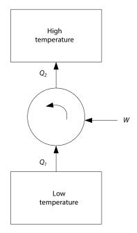
Figure 2.2: The reversed heat engine.
