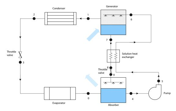
Figure 5.1: Vapour absorption cycle diagram.
