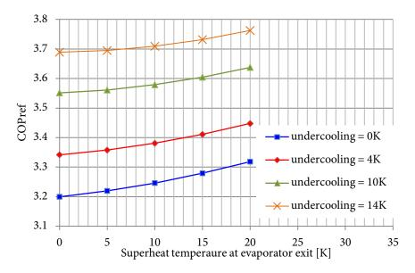
**Figure 7.9:** Refrigeration COP against superheat temperature at exit from the evaporator for various undercooling temperature at exit from the condenser.
