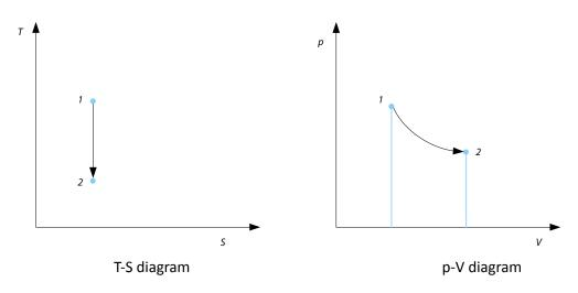
Figure 1.14: Isentropic process shown on a T-S and p-V diagram
