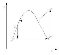
**Figure 4.3:** Modified Carnot cycle with under-cooled liquid at the condenser exit.
