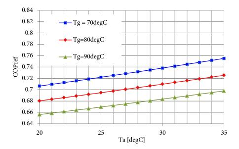
Figure 8.5: COP against absorber temperature.
