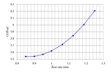
**Figure 7.11:** Refrigeration COP against mass flow rate ratio  $\dot{m}_{l'}/\dot{m}_{H'}$ . The evaporator pressure is set to 1.33 bar, the intermediate pressure at 6 bar and the high pressure condenser at 10 bar.
