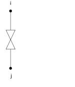
Figure 6.2: Throttle valve element.
