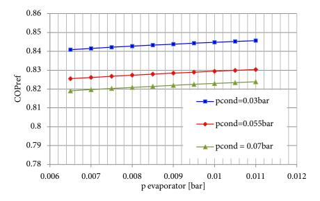
Figure 8.13: COP against evaporator pressure.
