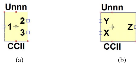
Figure 7.7: LTspice symbol for the current conveyor. Autogenerated from the netlist (a). Edited from the autogenerated symbol (b).
