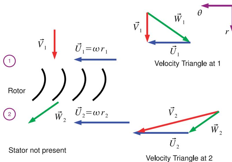
Figure 4.5: Velocity Triangles for a Radial Impeller
