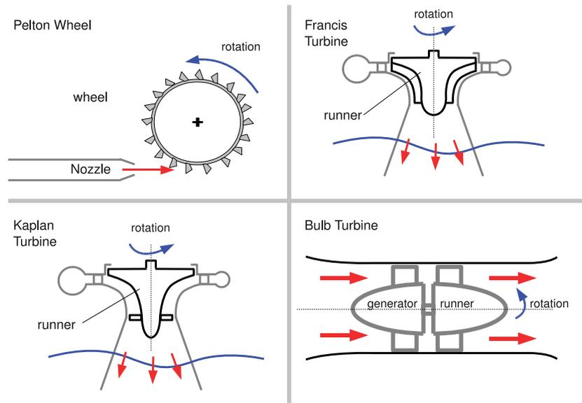
Figure 4.10: The Four Major Types of Hydraulic Turbine
