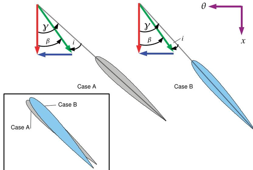
Figure 3.7: Schematic Showing Wind Turbine Pitch Control
