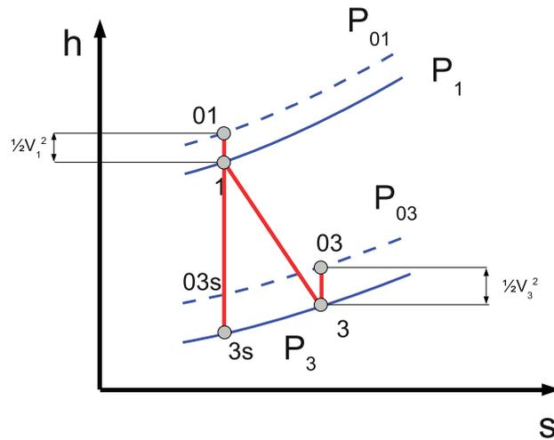
Figure 6.1: Enthalpy-Entropy Diagram for a Turbine
