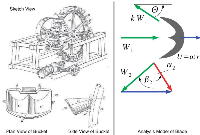
Figure 4.11: Pelton's Patent Application and Analysis Model
