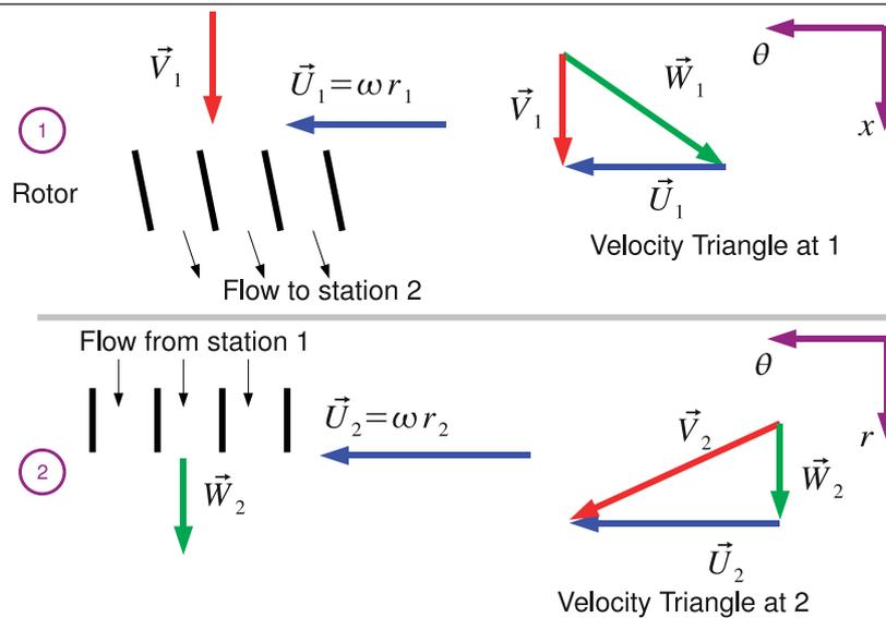
Figure 4.8: Velocity Triangles for a Centrifugal Impeller
