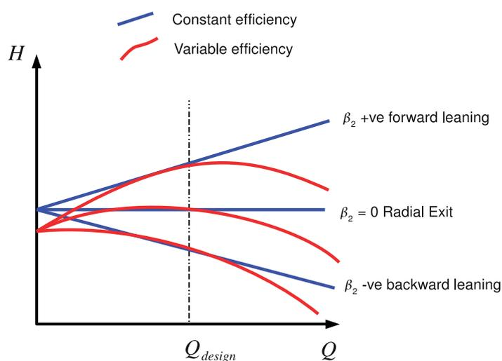
Figure 10.2:  $H$  vs  $Q$  for Three Blade Angles
