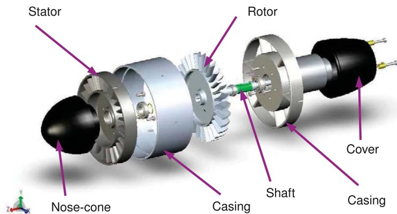
Figure 1.3: A Simple Turbine: Exploded View
