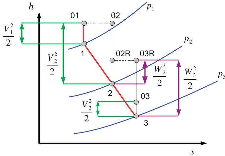
Figure 8.1: h-s diagram with  $h_0$  and  $h_{0rel}$
