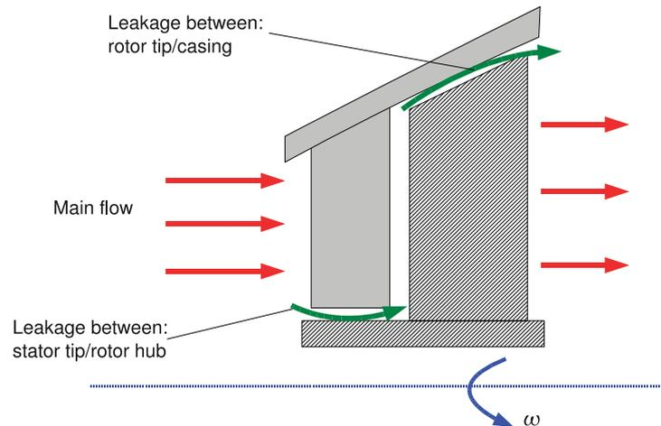
Figure 8.3: Locations for Tip Clearance Flow
