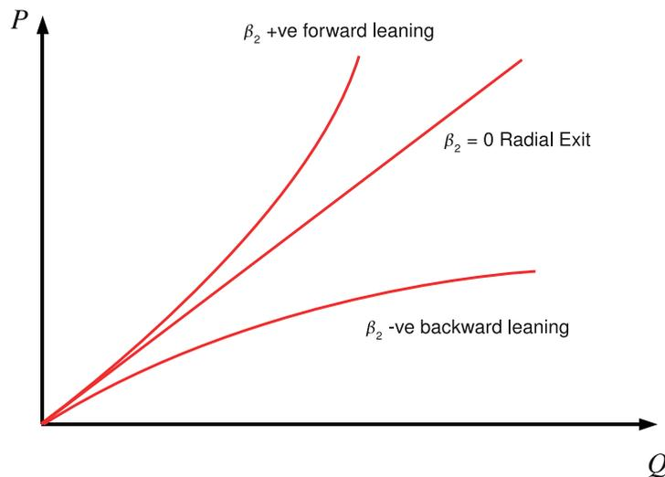
Figure 10.3:  $P$  vs  $Q$  for Three Blade Angles
