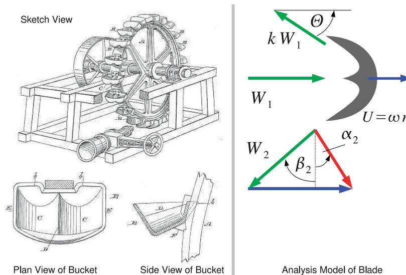
Figure 9.1: Pelton’s Patent Application and Analysis Model
