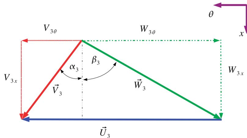
Figure 2.6: Velocity Triangles at Station 3 of a Turbine
