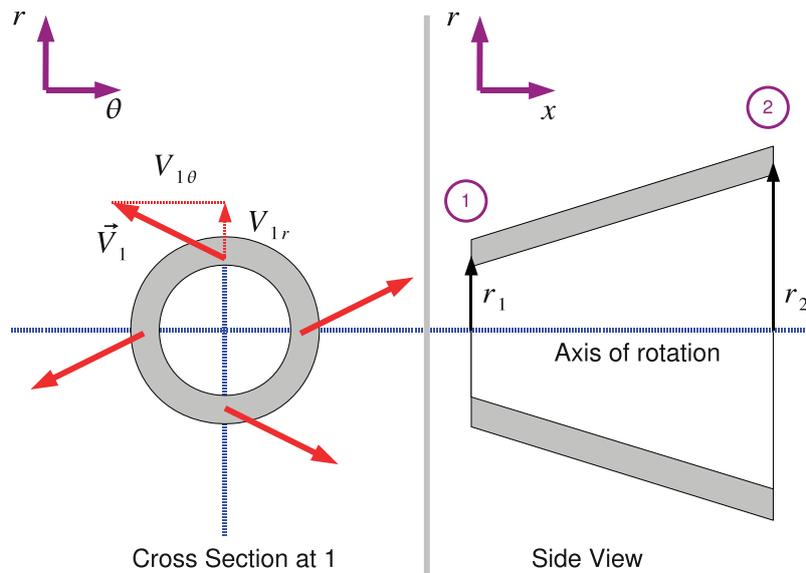
Figure 5.3: A Generic Turbomachinery Flow Passage
