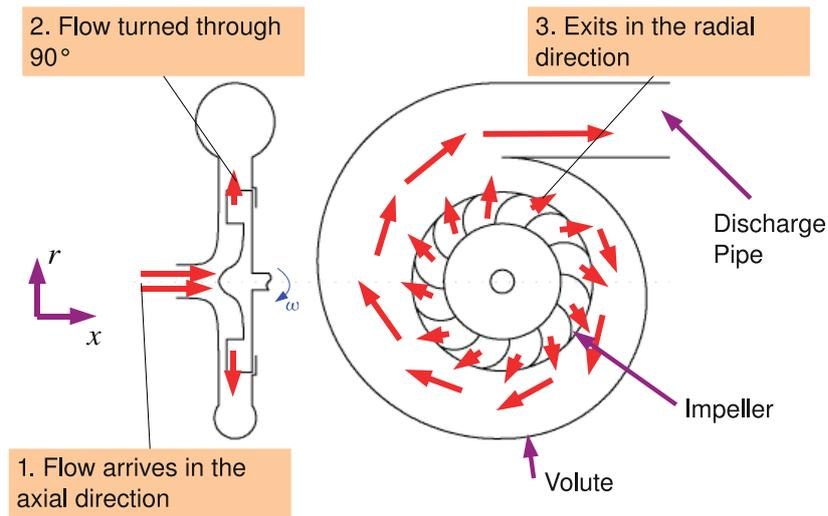
Figure 4.1: Radial Pump
