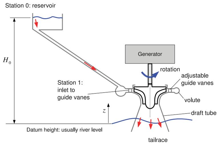
Figure 4.9: Schematic of Hydro-Electric Scheme
