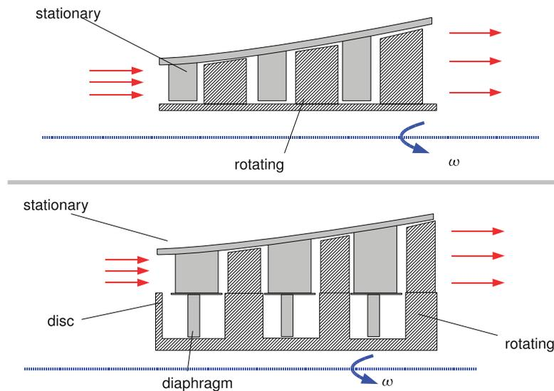
Figure 8.4: Schematics of Disc and Diaphragm Construction
