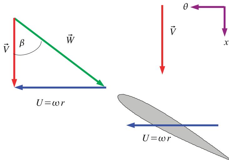
Figure 3.2: Wind Turbine Blade and Velocity Triangle
