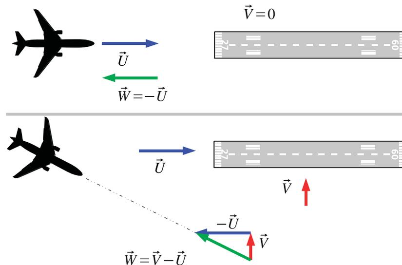
Figure 2.2: Velocity Triangles for an Aircraft Landing
