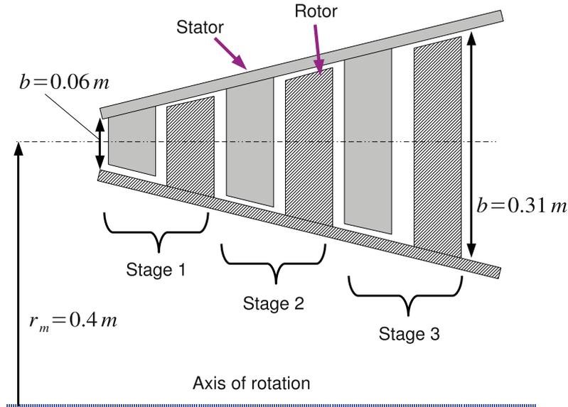
Figure 5.1: Meridional View of a Gas Turbine
