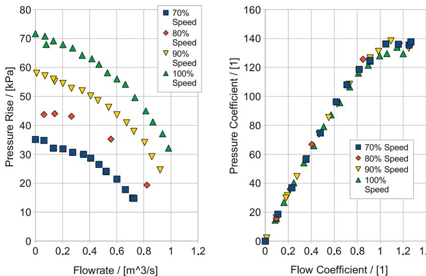
Figure 7.3: Collapsing Pump Data onto Non-dimensional Curves
