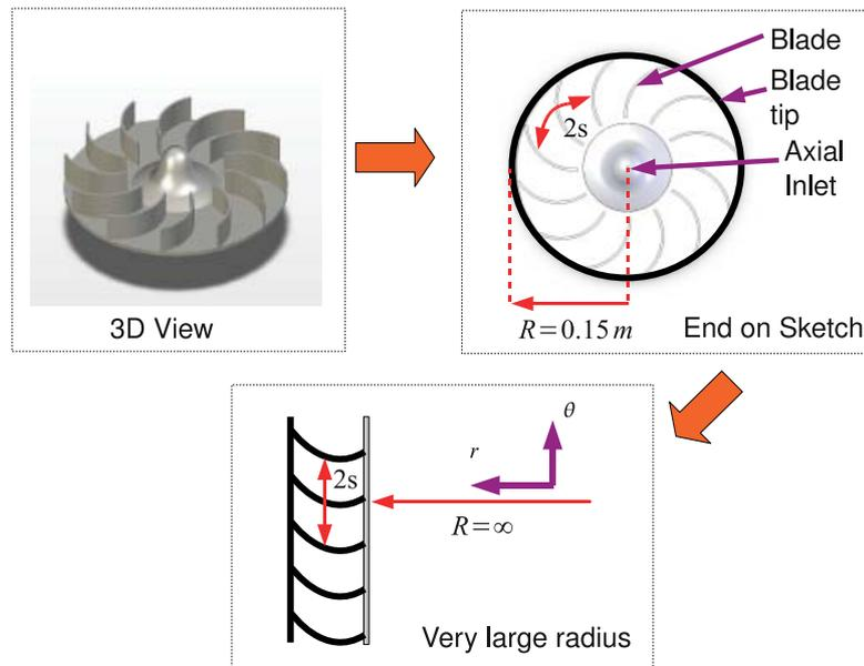
Figure 4.4: The Cascade View for a Radial Impeller
