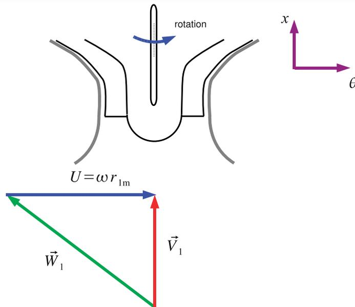
Figure 10.4: Inlet to Pump Impeller
