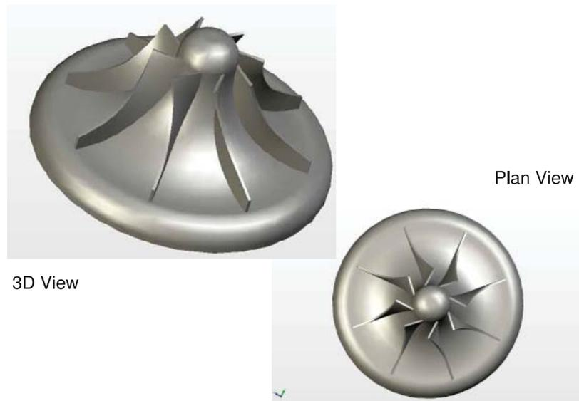
Figure 4.3: Centrifugal Impeller
