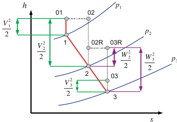
Figure 6.5:  $h$ - $s$  diagram with  $h_0$  and  $h_{0rel}$
