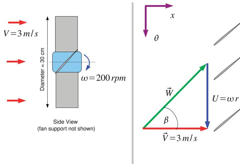
Figure 2.7: Velocity Triangles for a Desk Fan
