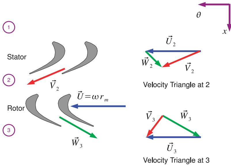
Figure 2.5: Velocity Triangles for a Turbine Stage
