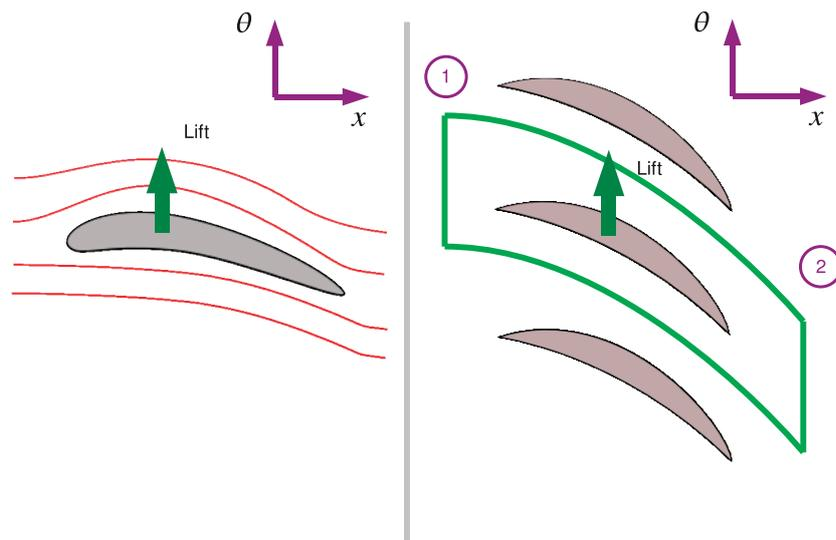
Figure 5.4: Isolated Aerofoil compared to a Cascade
