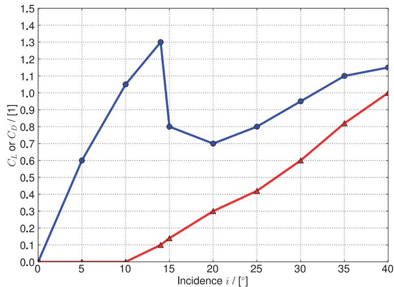
Figure 3.5:  $C_L$  and  $C_D$  for a NACA 0012 Aerofoil
