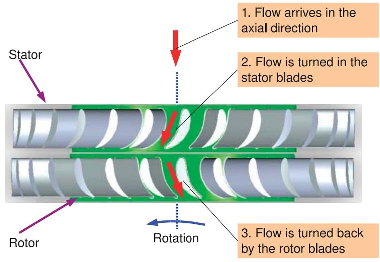
Figure 1.4: Simple Turbine Operation
