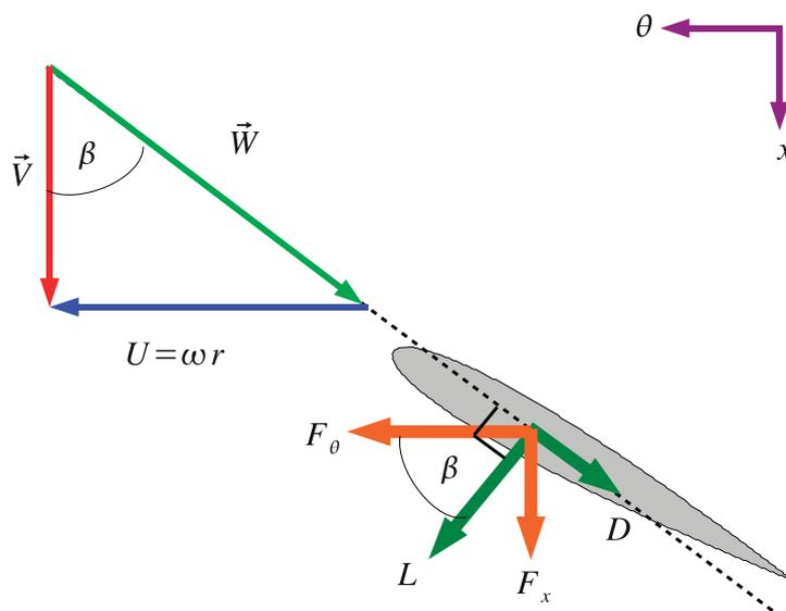
Figure 3.3: Forces on a Wind Turbine Blade
