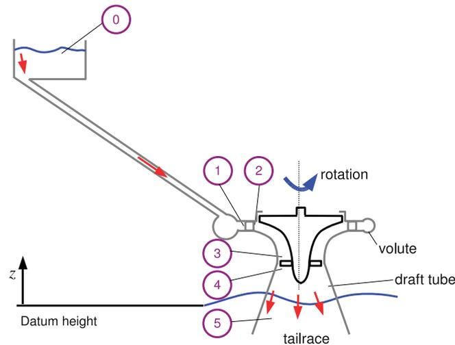
Figure 9.5: Analysis of a Kaplan Turbine
