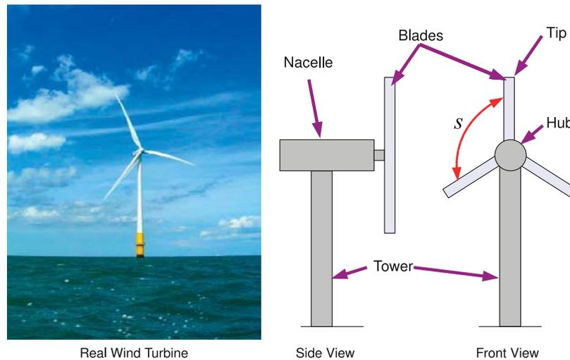
Figure 3.1: Wind Turbine Picture and Sketch
