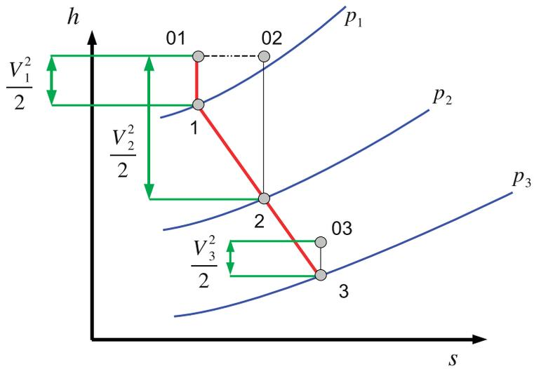
Figure 6.4: h-s diagram with  $h_0$
