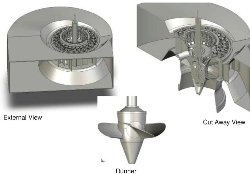
Figure 4.13: Three Dimensional Views of a Kaplan Turbine
