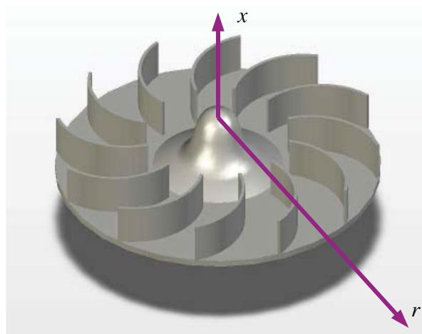
Figure 4.2: 3D View of the Radial Impeller
