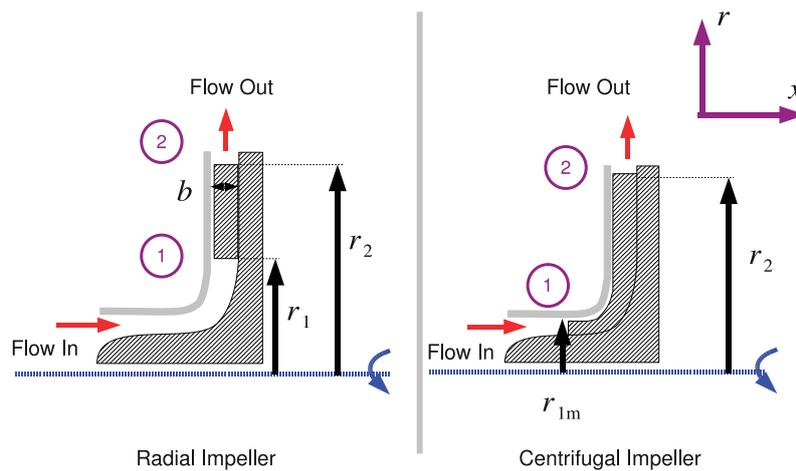
Figure 5.2: Meridional Views of Radial and Centrifugal Machines
