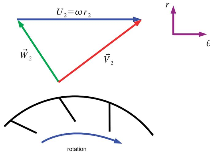
Figure 10.5: Exit from Pump Impeller
