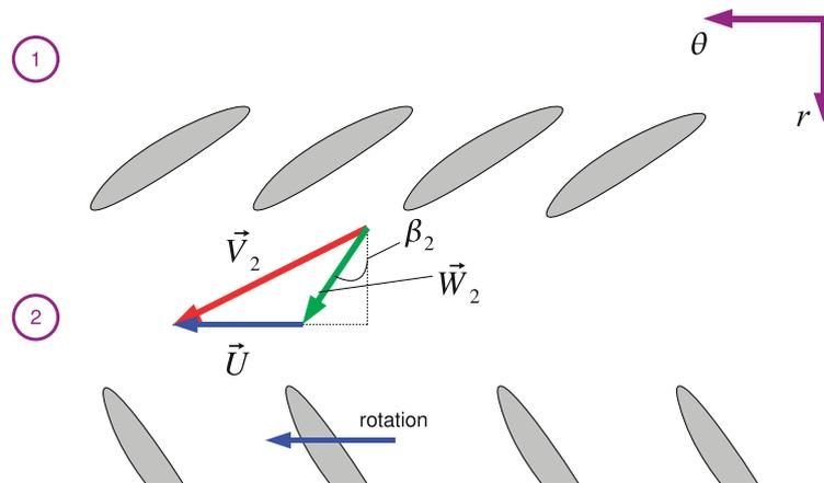
Figure 9.3: Velocity Triangle for Francis Turbine Guide Vane Exit
