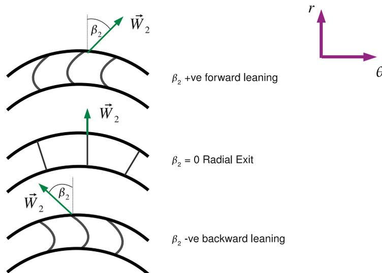
Figure 10.1: Three Blade Angles at Impeller Exit
