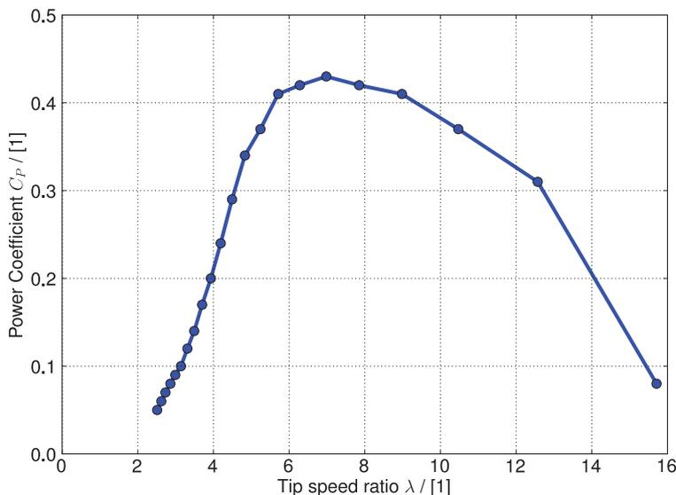
Figure 7.2:  $C_P$  vs  $\lambda$  for 2.5MW Wind Turbine
