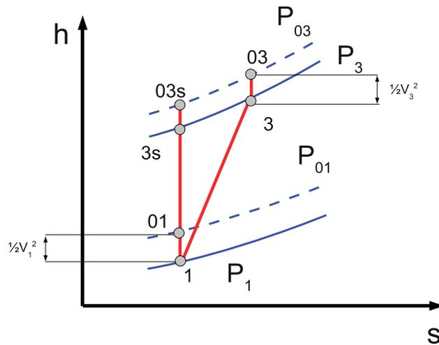
Figure 6.2: Enthalpy-Entropy Diagram for a Compressor
