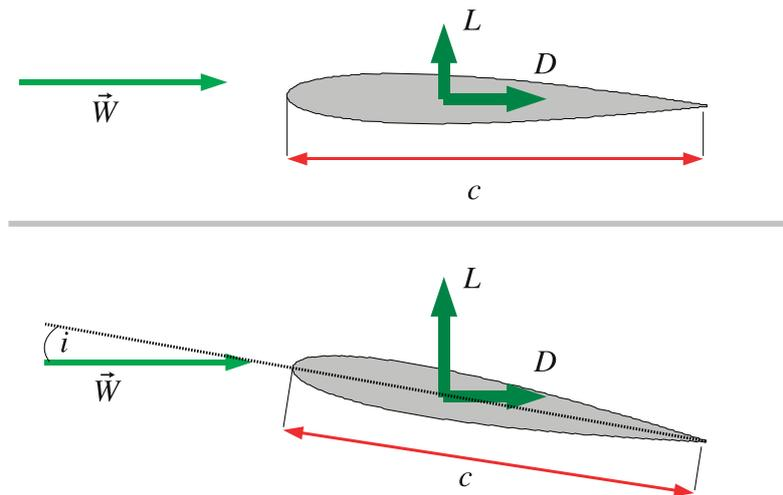
Figure 3.4: Aerofoil at Two Incidences
