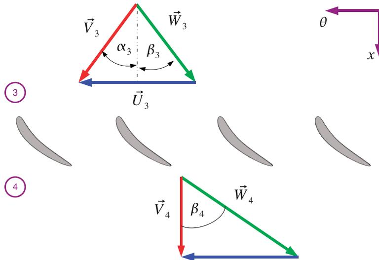
Figure 9.7: Velocity Triangle for a Kaplan Runner
