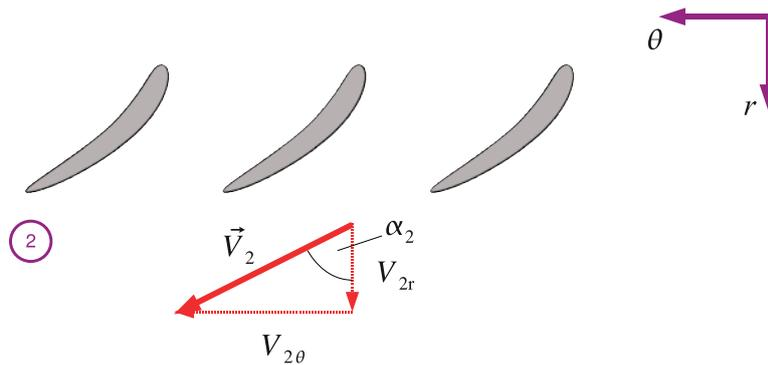
Figure 9.6: Velocity Triangle for a Kaplan Turbine at Guide Vane Exit
