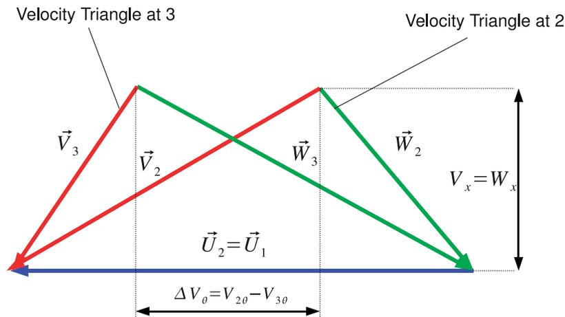
Figure 7.1: Velocity triangles for exit and inlet combined
