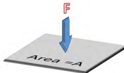
Figure 2.1. Definition of pressure. Force F acting on an area of A \text{ m}^2 .
