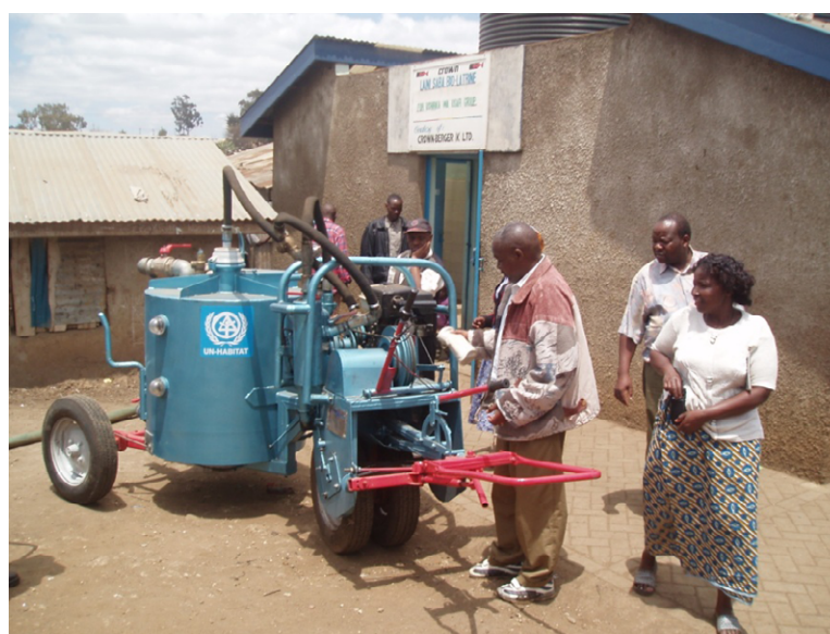
Figure 3.9: The ‘Vacutug’ developed by UN-Habitat.
