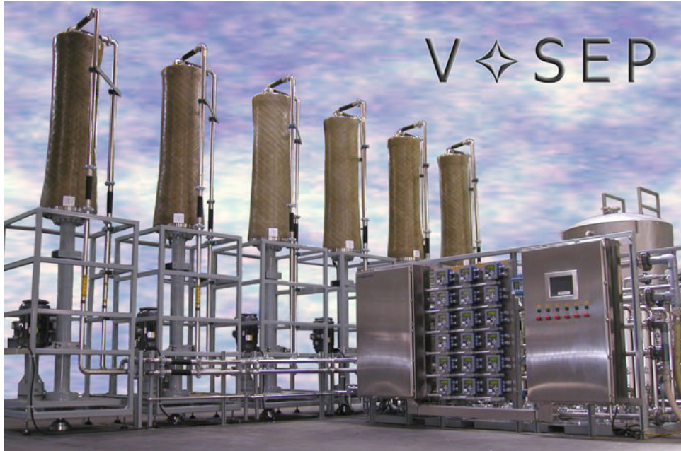
Fig 23. Industrial VSEP modules with 150 m 2 of membranes
