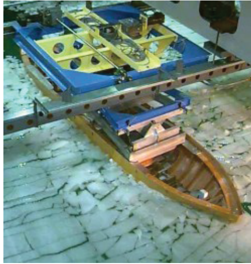
Figure 4.3: Model test with PMM in ice performed by Oceanic Consulting Corporation (see 1 (n.d.a))
