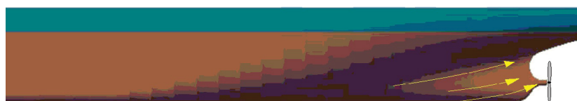
Figure 7.7: Upward oblique flow in the ship stern area (side view)
