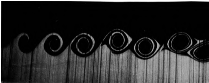
Figure 9.13: Development of instability in the free jet.
