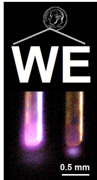
Figure 8-1. Hydrogen diffusion microflames near their quenching limits (Lecoustre et al., 2010): in air (left) and in oxygen (right). A shutter time is 30 s.
