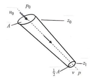
The flow is represented in the figure; to proceed, we first use mass conservation in the form: speed×area = constant i.e.  $Au_0 = \frac{1}{2}Av$  so  $v = 2u_0$ . Now we apply Bernoulli's equation along a streamline associated with the flow through the pipe:
