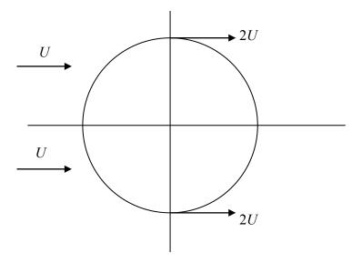
We now take this investigation one step further by calculating the pressure distribution around the circle. Let us assume that there are no body forces, and that the pressure at infinity is  $p_0$ ; remember that the flow is incompressible and, we have argued, body forces are negligible in the flows that we wish to examine. We apply Bernoulli's equation to the streamline that comes from infinity, goes around the circle and then moves off (to the right) back to infinity; thus we obtain
