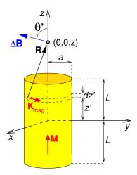
(a) Because the magnetisation field is uniform, there is no magnetisation volume current. The magnetisation surface current  $\mathbf{K}_{\text{mag}}(\mathbf{r}) = \mathbf{M}(\mathbf{r}) \times \hat{\mathbf{n}}$  is zero on the two ends, and  $\mathbf{K}_{\text{mag}}(\mathbf{r}) = M_0 \hat{\boldsymbol{\phi}}$  on the cylindrical surface.
