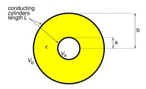
(a) We start by solving Laplace's equation in cylindrical coordinates with no dependence on  $\phi$  and z
