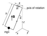
(a) Assuming the position of the pendulum mass is still described by  $\mathbf{r}_m(t) \approx h \theta_0 \cos(\omega t) \hat{\mathbf{x}}$ , what is the magnetic flux  $\Phi_B(t)$  through the circuit, and hence the emf as a function of time? Take the direction around the circuit indicated by the arrow to correspond to positive emfs and currents.
