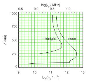
(b) Reading off the plot, we obtain the height of the reflecting layer shown in the table below.
