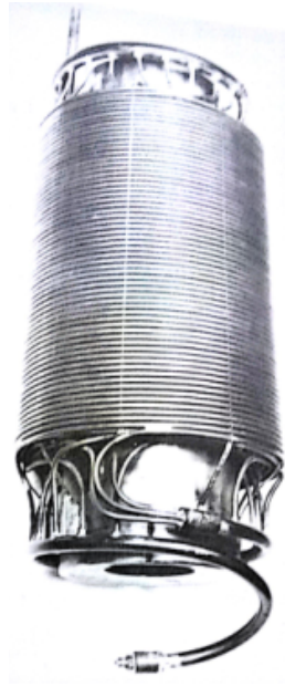
Fig. Giaque-Hampson heat exchanger, with the outer shell and insulation removed.
