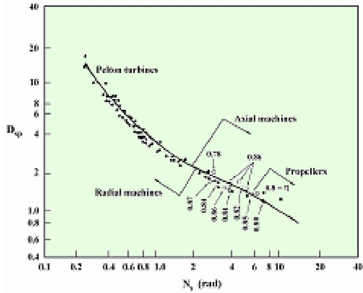
Fig. 2.9 "Cordier" line in  $N_s$ ,  $D_{sp}$  diagram
