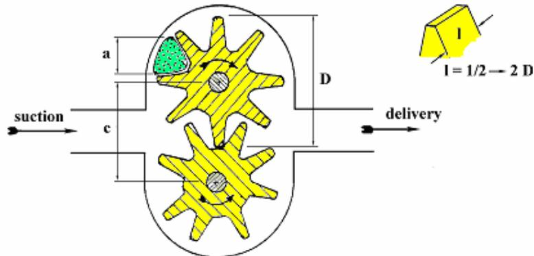
Fig. 8.9 Gear wheel pump
