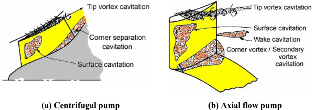
**Fig. 3 Location of cavitation in centrifugal and axial flow pumps**
