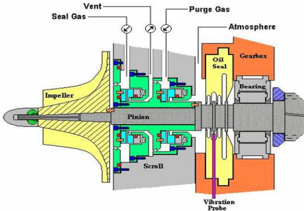
**Fig. 4.14 Tandem mechanical seal, type B, with degassing chamber and flow-inducing ring at the secondary seal**
