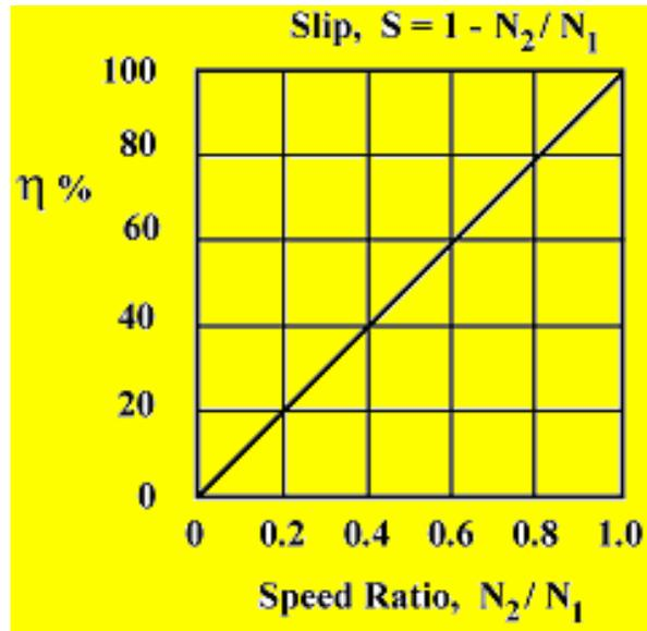
**Fig. 5.36 Fluid coupling efficiency curve**
