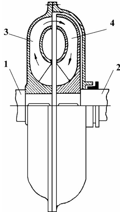
**Fig. 5.35 Fluid coupling**
