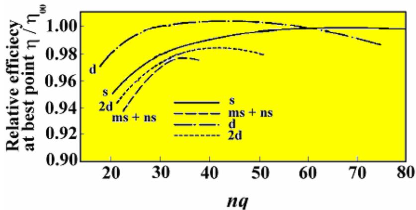
$$nq = n \cdot Q^{1/2} / H^{3/4} \text{ where } Q \text{ (m}^3/\text{s), } H \text{ (m), and } n \text{ (min}^{-1}\text{)}$$
