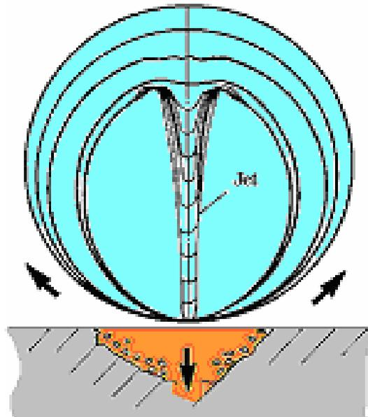
**Fig. 7 (a) The jet collapse model for damage due to cavitation**
