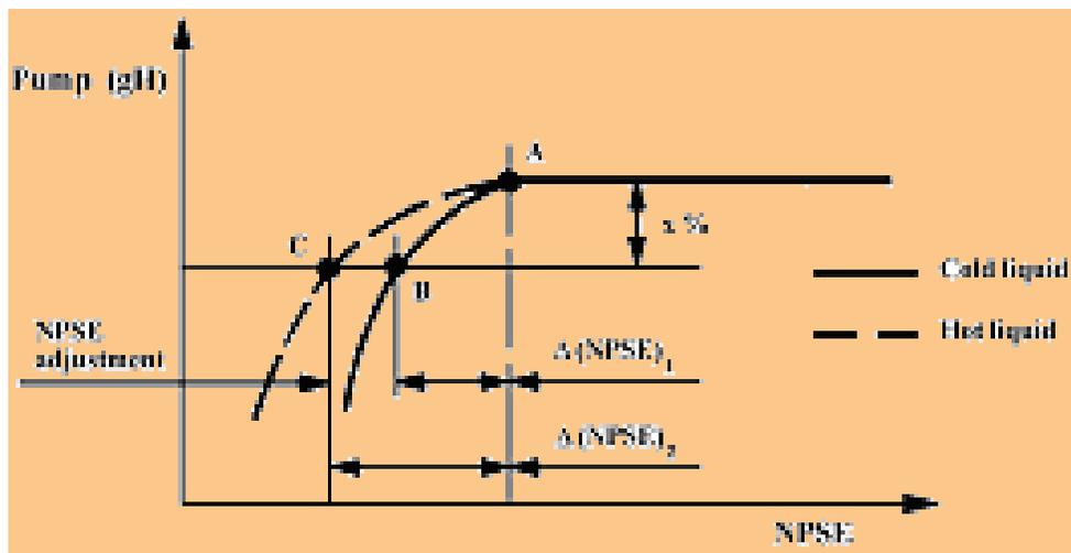
Fig. 10 The variation on NPSE required of liquid temperature
