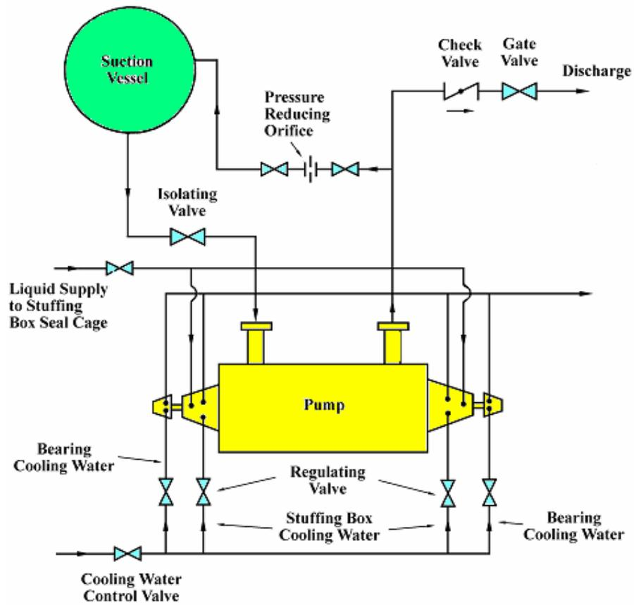
**Fig. 4.46 Example for auxiliary and main piping of a centrifugal pump (Worthington Corp.)**
