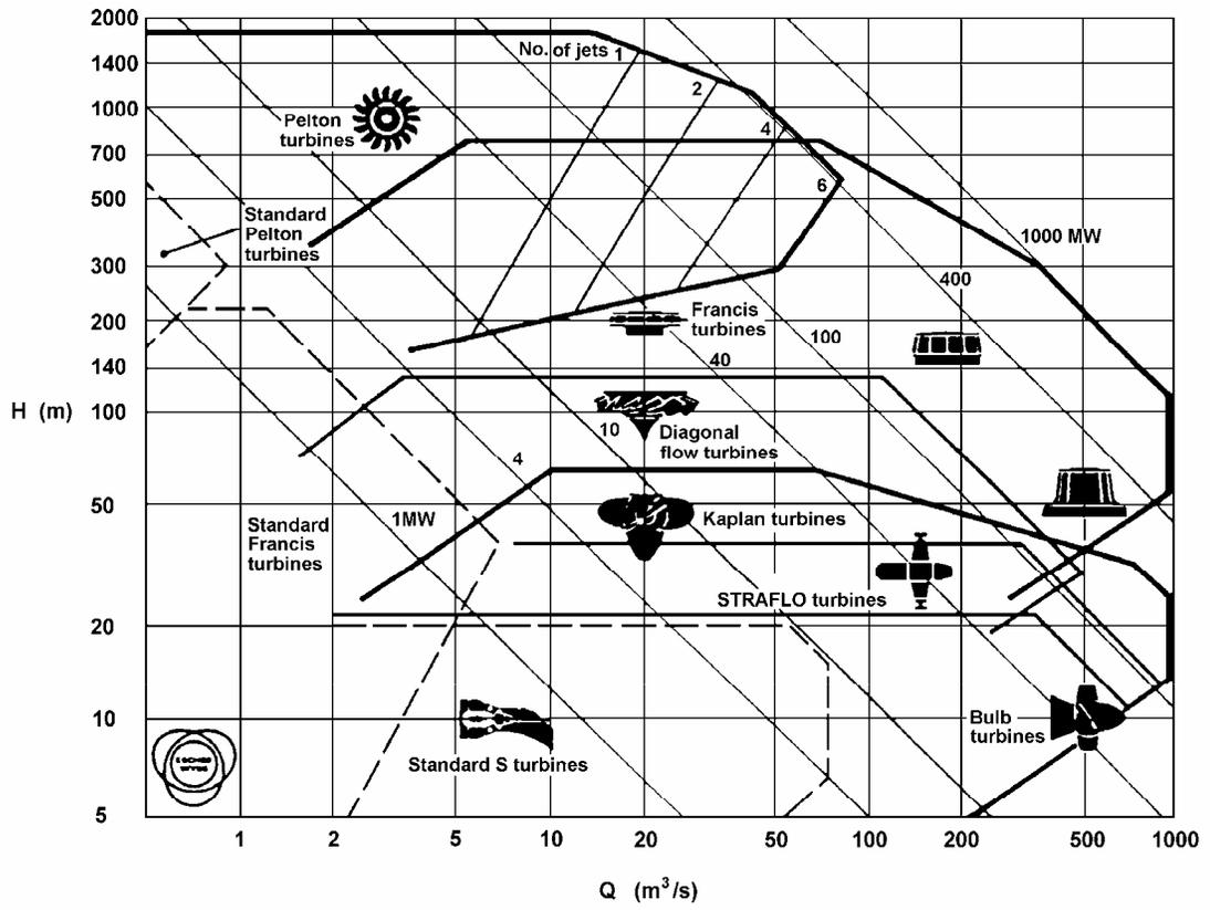
Fig. 5.41 Application ranges of different types of water turbines
