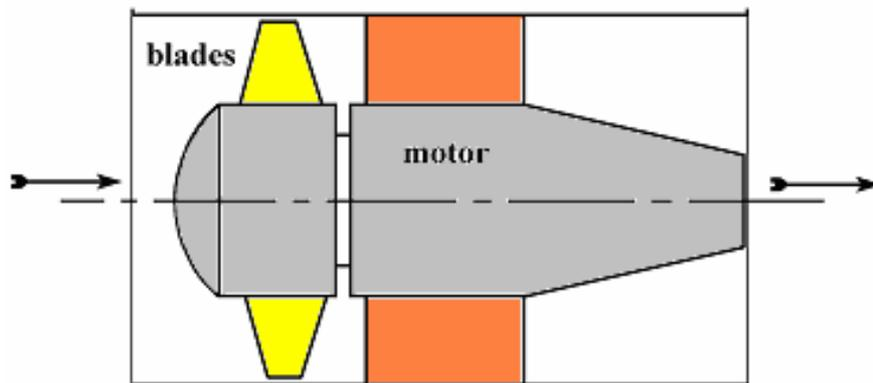
Fig.7.1 Fan with the driving motor
