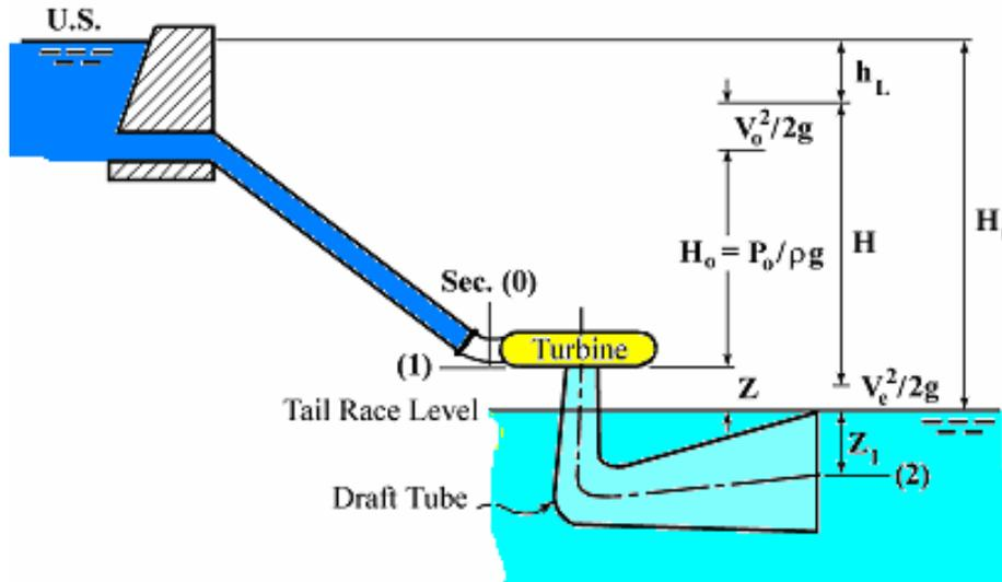
**Fig. 5.16 Schematic diagram of reaction turbine installation**
