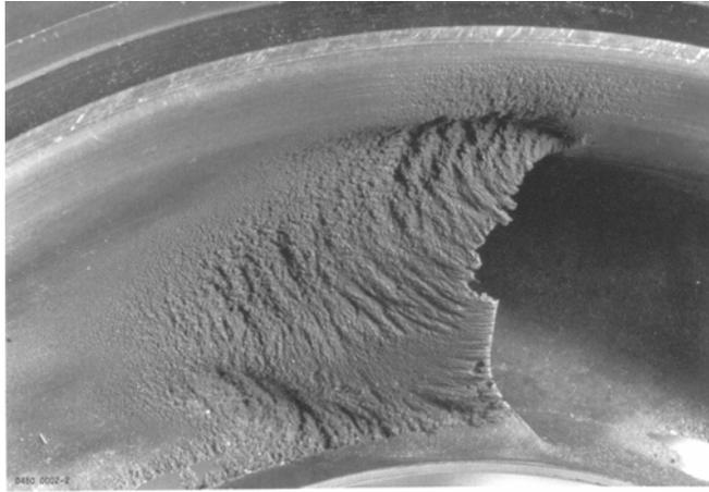
**Fig. 25 Pump impeller showing cavitation erosion**
