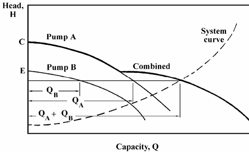
Fig. 4.30 Pumps in parallel
