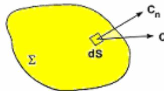
**Fig. 1.4 The surface element**
