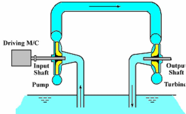
Fig. 5.34 The principles of hydraulic transmission
