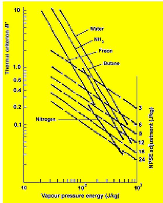
**Fig. 11 Plot of thermodynamic adjustment factors (from Stahl and Stepanof, 1956)**
