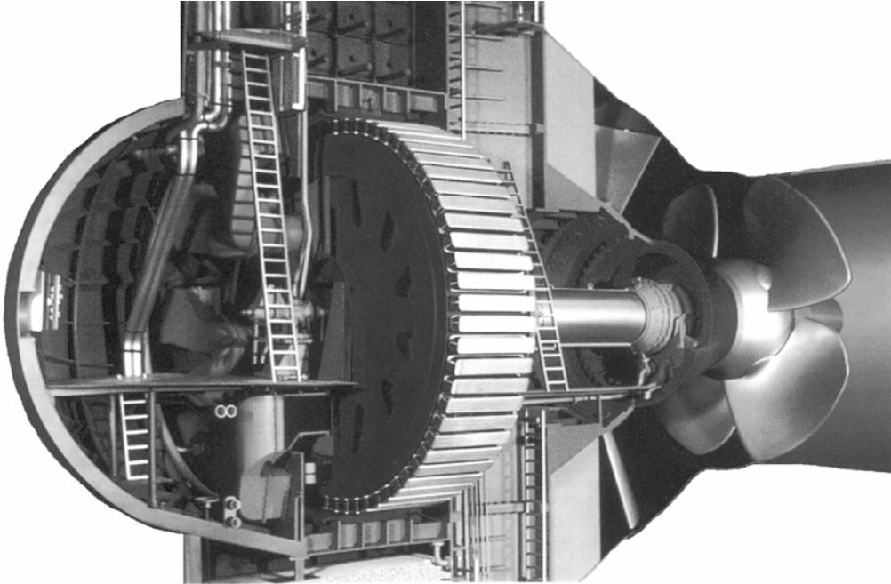
**Fig. 5.46** The six bulb turbines at Vienna's Freudenau power plant belong to the largest one world-wide
