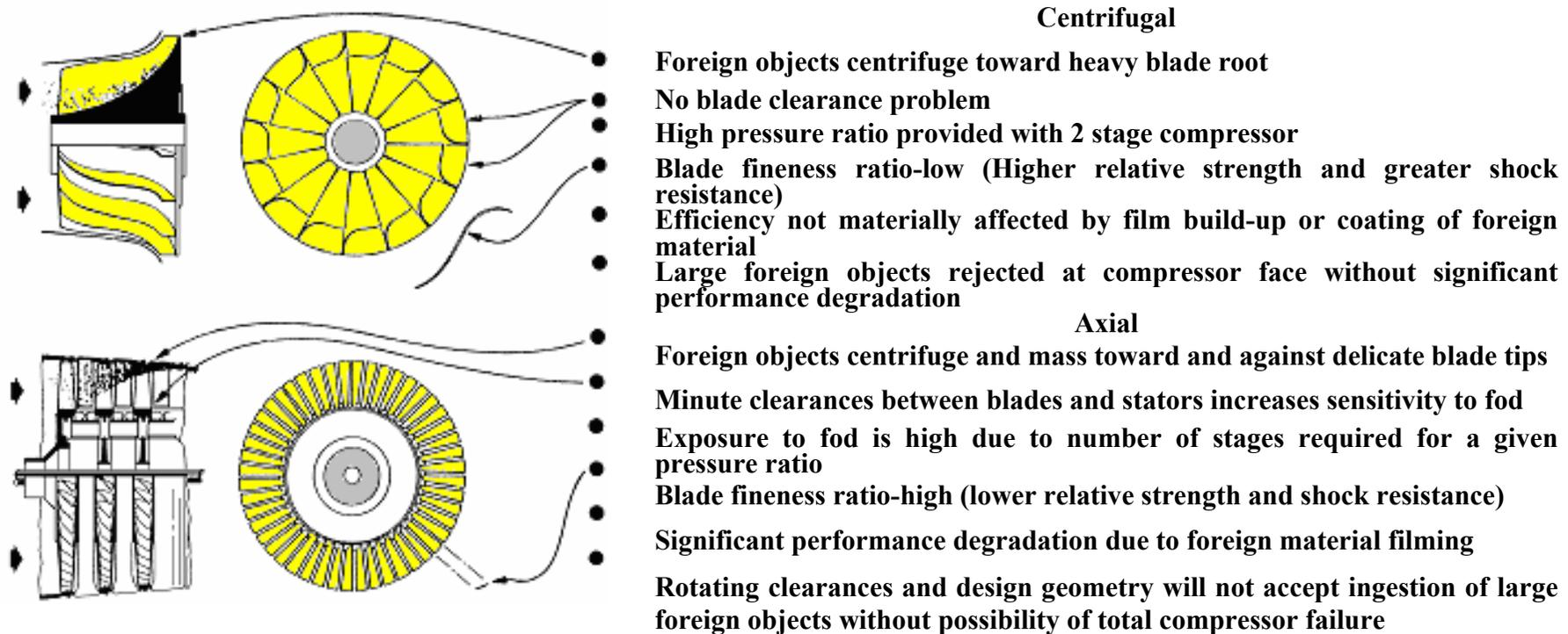
**Fig. 7.15 Compressor air flow patterns
