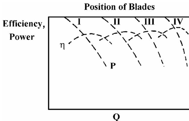
**Fig. 4.28 Performance curves for variable pitch axial pump**
