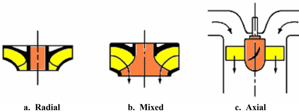
Fig. 5.9 Reaction turbine runners
