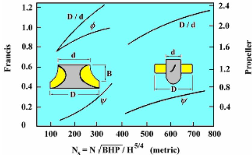
Fig. 5.25 Design characteristics for Francis and propeller turbines
