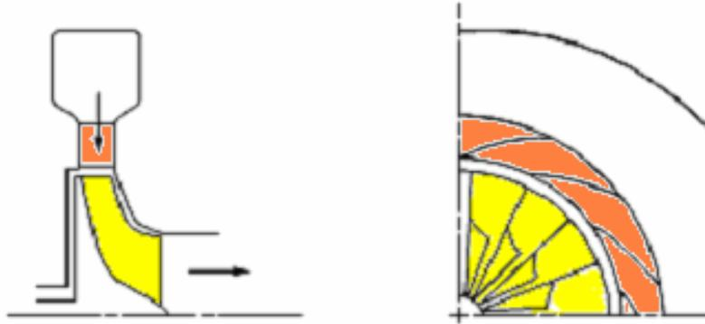
**Fig. 5.11 Typical radial inward flow turbine profile**
