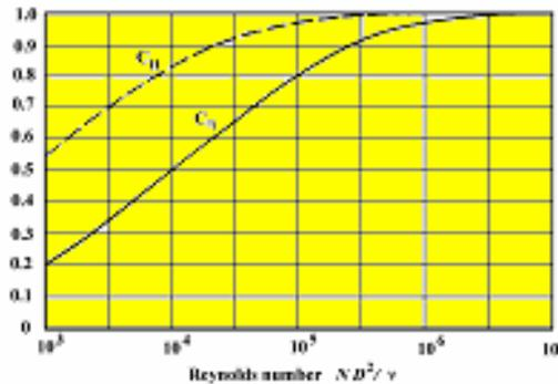
**Fig 2.3 Reynolds Number factor for head  $C_H$  and efficiency  $C_\eta$**
