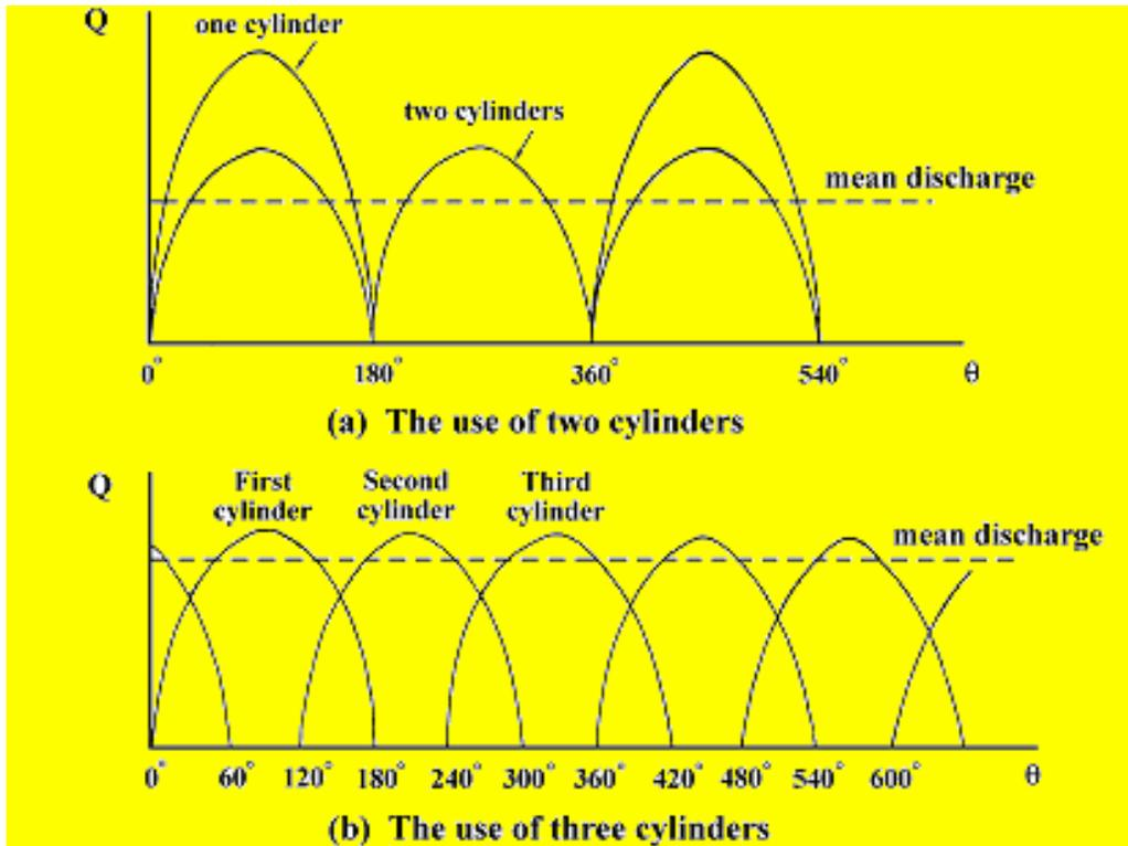
Fig. 8.4 The damping of fluctuation
