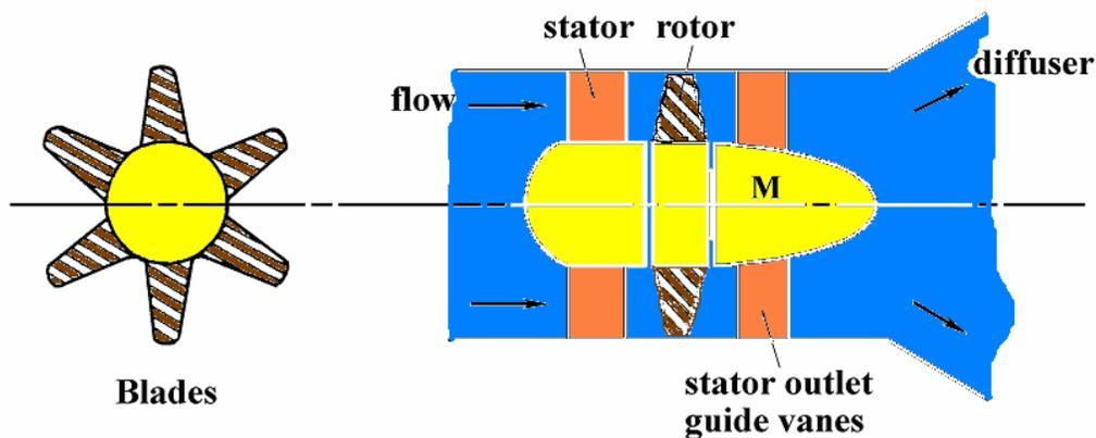
Fig. 4.21 Propeller pump
