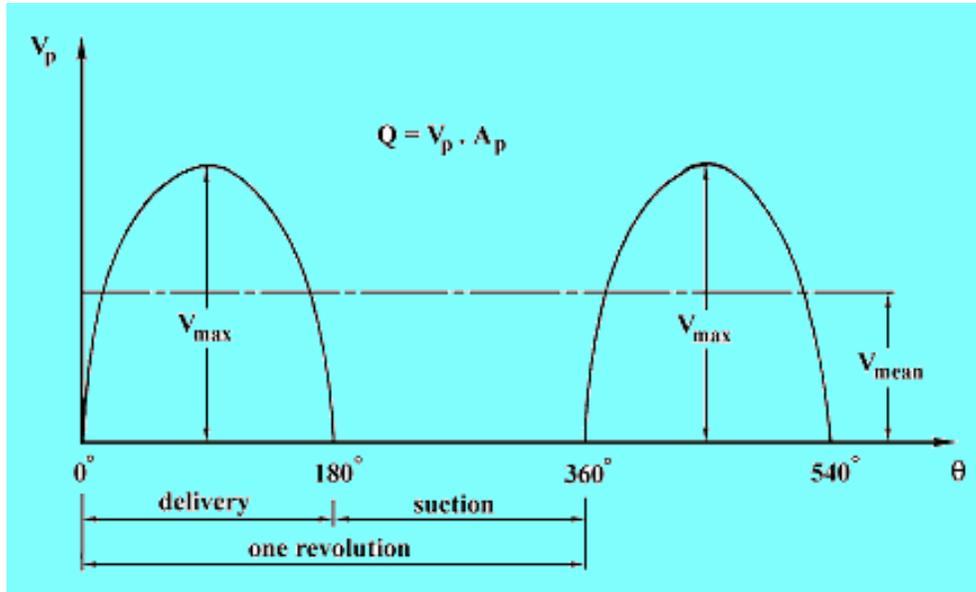
**Fig. 8.2 The instantaneous velocity in delivery pipe**
