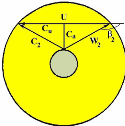
Fig. 5 Velocity triangle at diffuser inlet
