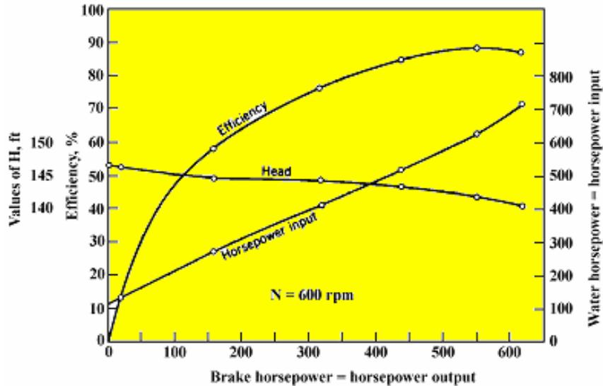
Fig. 5.22 Performance at constant speed and variable gate opening
