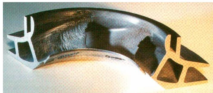
Fig. 24 Sheet and groove erosion on a pump impeller
