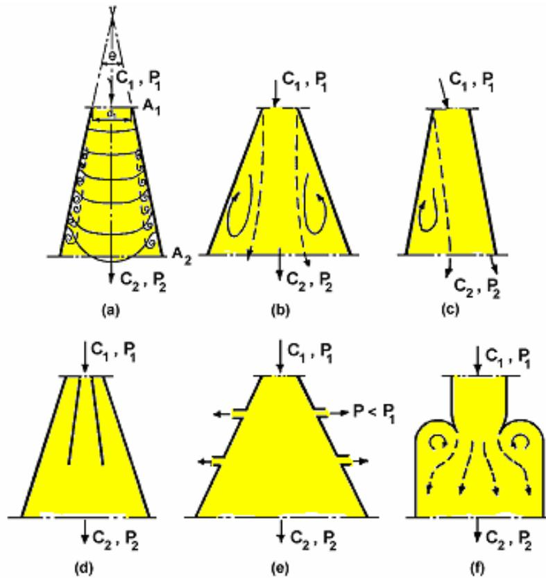
**Fig. 1 Diffuser. (a) Boundary-layer increase in diffuser. (b) and (c) Stall zones. (d) Short vane dividers. (e) Boundary-layer absorption. (f) Diffuser with standing vortices.**
