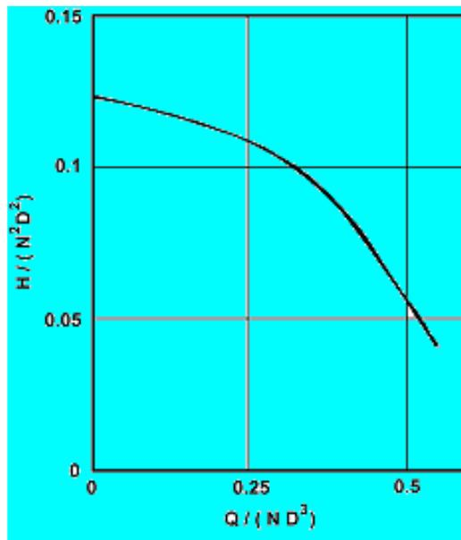
Fig. 2.1 Non-dimensional Head-Volume characteristics
