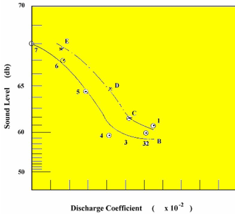
**Fig. 26 Sound level at frequencies 28600 and 14300 CPM at impeller speed equals 2860 (5 blades)**
