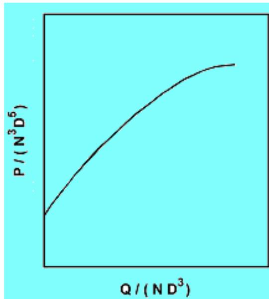
Fig 2.2 Non-dimensional Power-Flow characteristics
