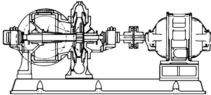
**Fig. 4.56 Centrifugal pump and motor placed on a large sub-base and connected by a suitable coupling for direct-drive**
