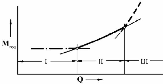
**Fig. 4.33** Minimum submergence  $M_{req}$  as a function of the flowrate
