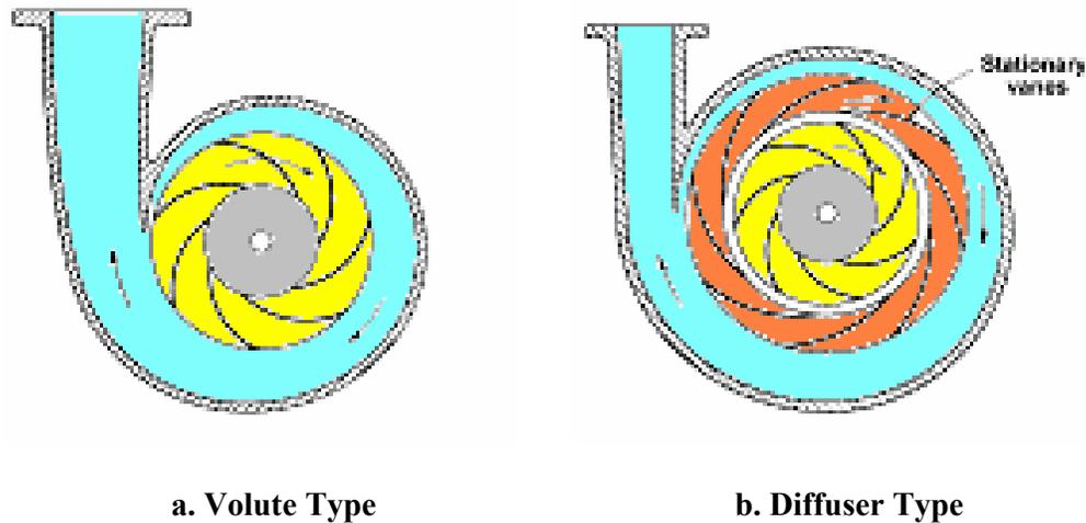
**Fig. 4.2 Centrifugal pump types**
