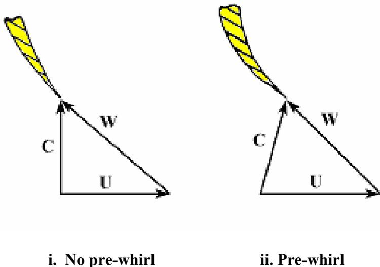
Fig. 7.9 The pre-whirl tends to reduce the relative velocity  $W$
