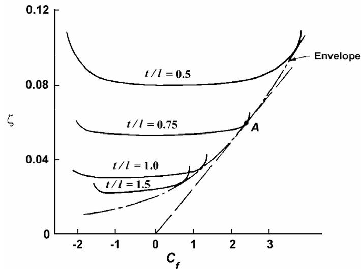
**Fig 3.6 Loss-coefficient versus tangential force coefficient curves of cascades (adapted from Csanady)**
