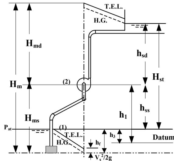
**Fig. 12 Schematic Diagram of Pump Installation**
