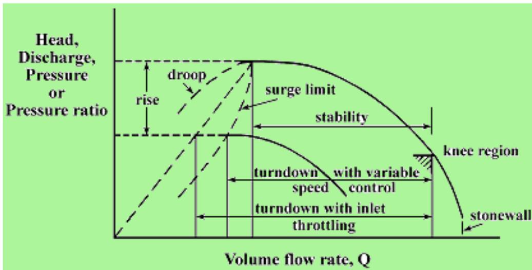
Fig. 7.7 Centrifugal compressor performance curve
