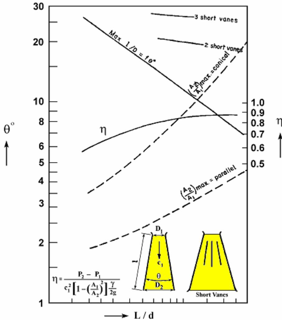
Fig. 2 Angle of divergence  $\theta$  of diffusers versus  $L/D$  (at stall limits) and recovery value  $\eta$ . (Based on test result reported by Kline)
