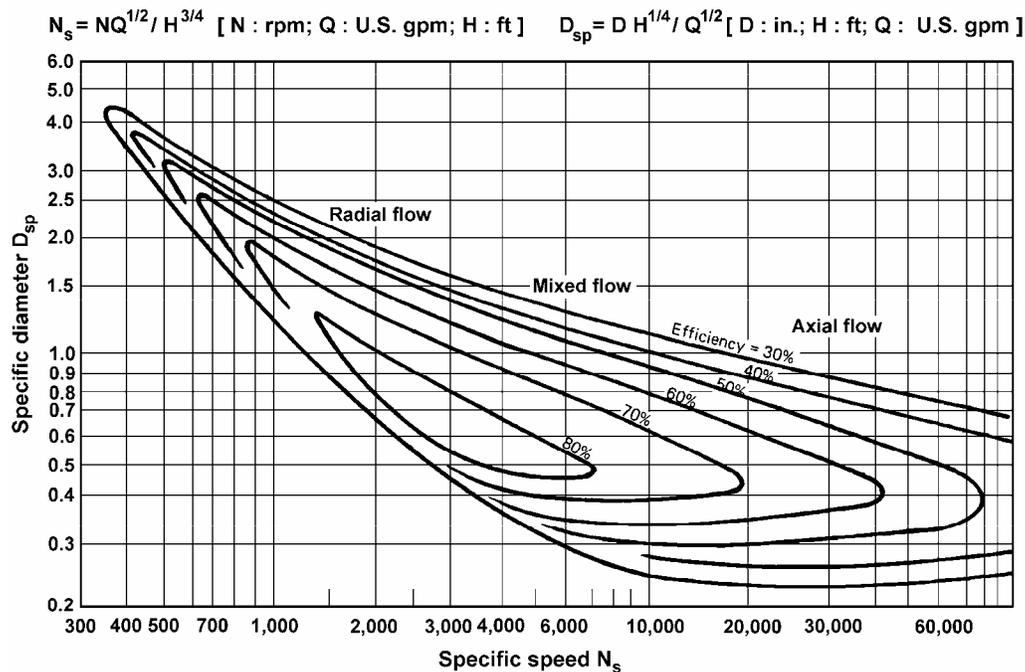
Fig. 4.29 Specific speed chart for the preliminary selection of single speed centrifugal pumps
