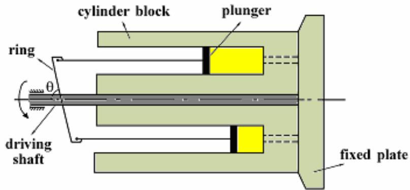
Fig. 8.8 Parallel cylinder rotary pump
