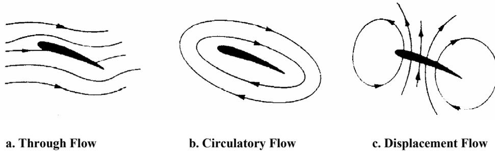
Fig. 3.12 Flow around a moving blade profile
