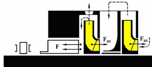
c. Balance Device with Balance Piston and Thrust Bearing
