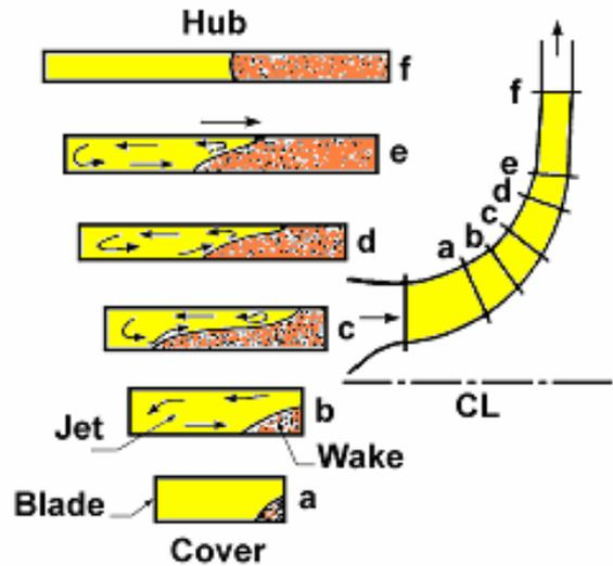
**Fig. 1.8 Development of the wake, secondary flow pattern
