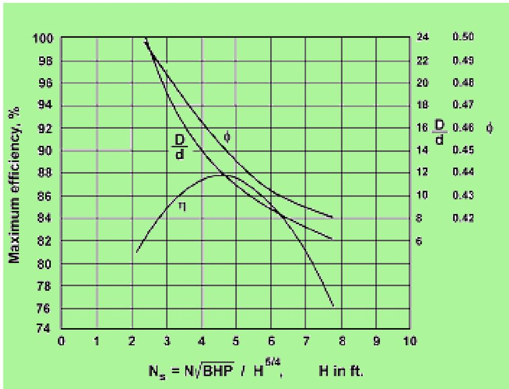
Fig. 5.8 Relation between  $\phi$ ,  $N_s$  and  $D/d$
