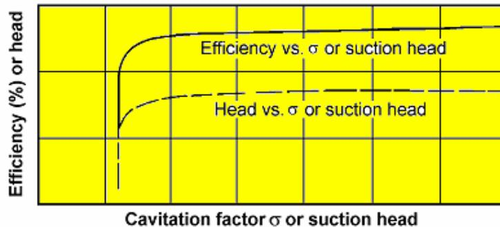
**Fig. 5 (b) Cavitation characteristics at constant speed and capacity**
