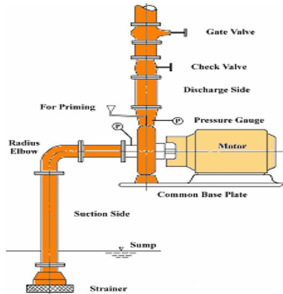
Fig. 4.42 Actual pump installation
