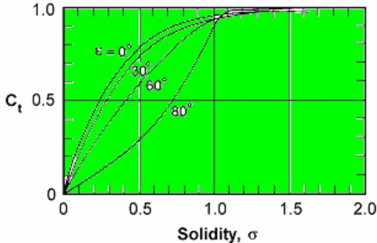
**Fig. 3.19 Coefficient  $C_t$  versus solidity for various stagger angles of a cascade of flat plates**
