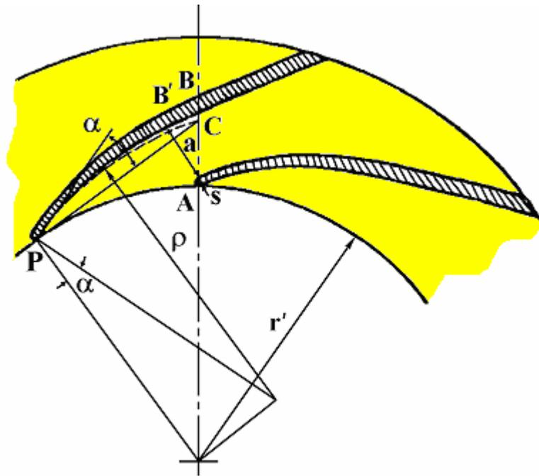
**Fig. 7 Logarithmic spiral and its radius of curvature as guide blade inlet**
