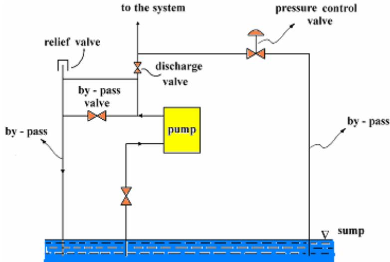
Fig. 8.6 Typical positive pump installation
