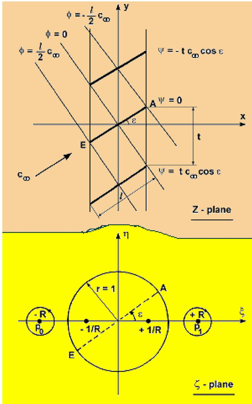
Fig. 3.17 Conformal transformation of a flat plate cascade
