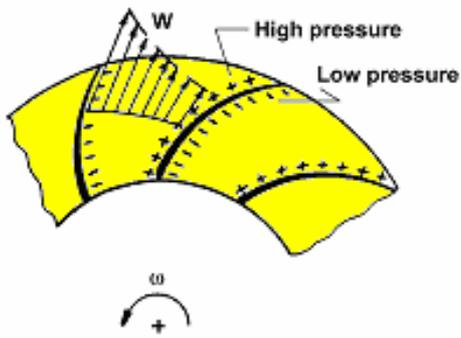
**Fig. 1.6 Pressure distribution between two blades**
