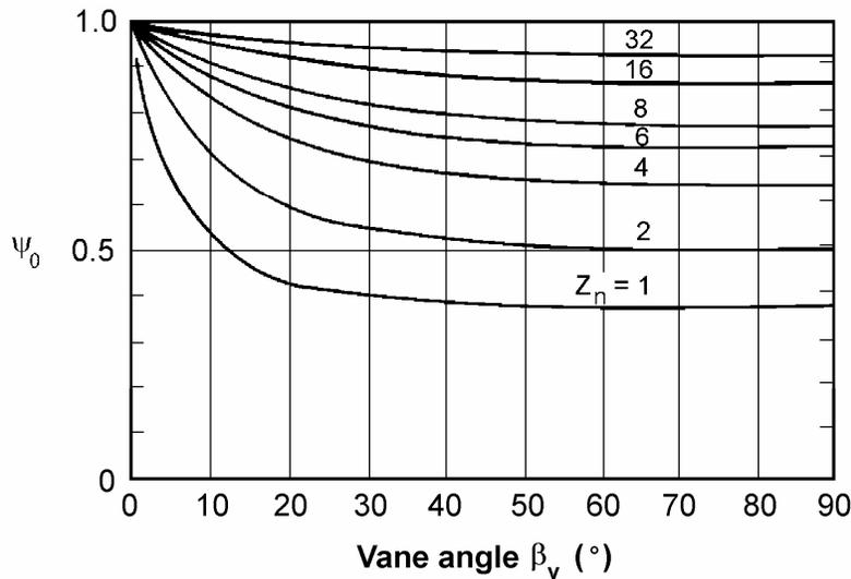
**Fig. 3.20 Values of shut-off head coefficient  $\psi_o$  for various vane angles  $\beta_v$  and number of vanes for a radial cascade of logarithmic spiral blades**
