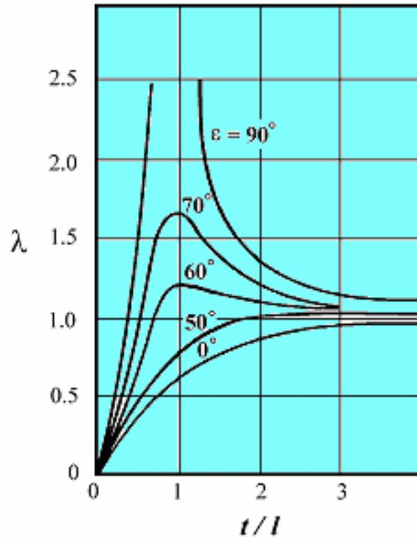
**Fig. 3.18 Theoretical lift ratio for flat plate cascade versus pitch chord ratio for different stagger angles**
