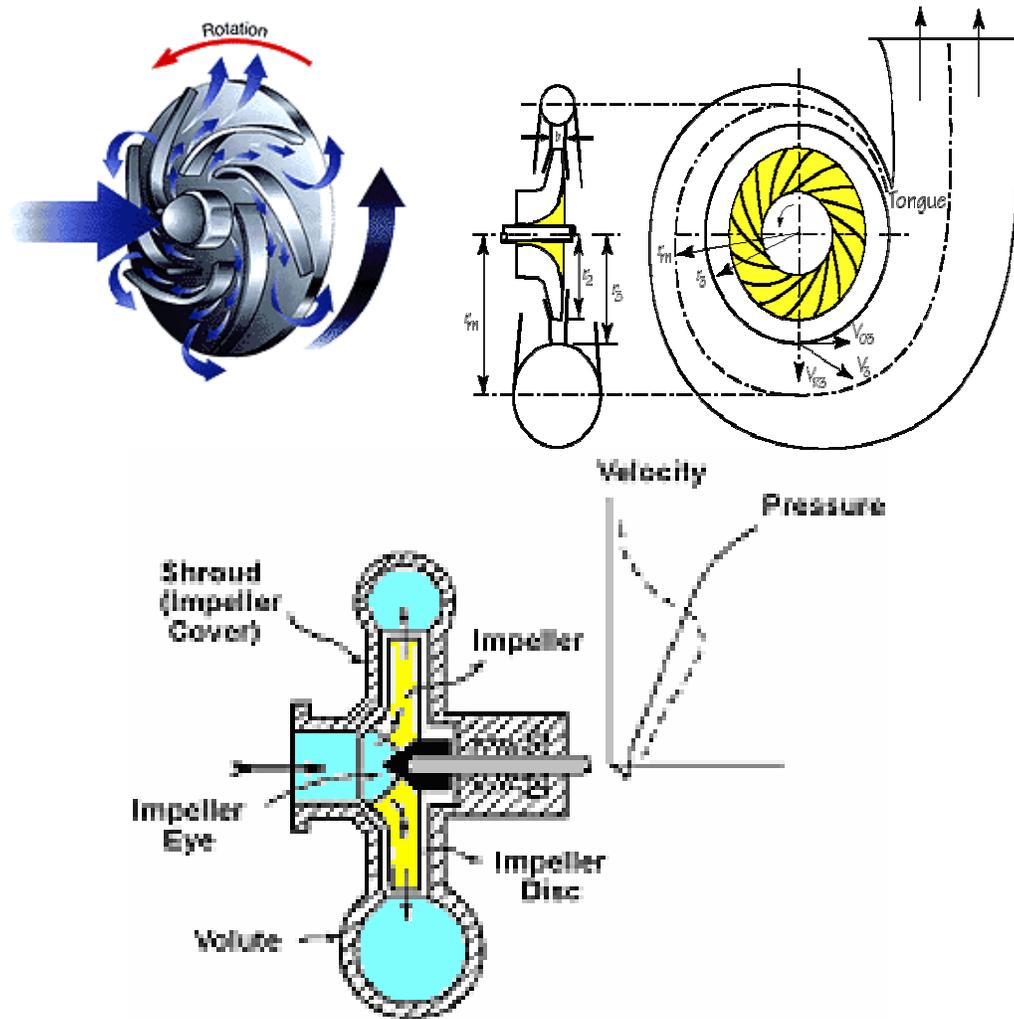
Fig. 4.1 Section at centrifugal pump
