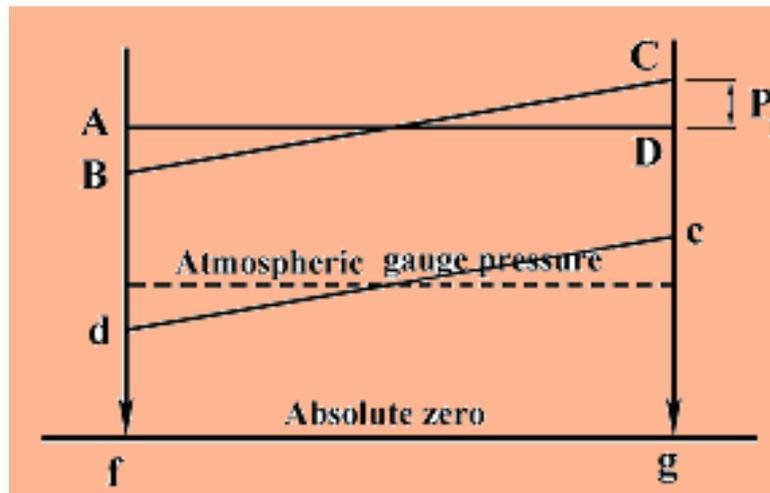
Fig. 8.12 Pressure in delivery line
