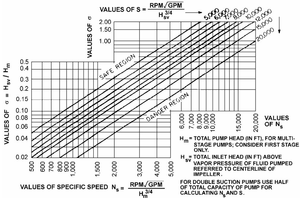
**Fig. 13 Cavitation limits of centrifugal and propeller pumps (Worthington Pump and Machinery Corporation)**
