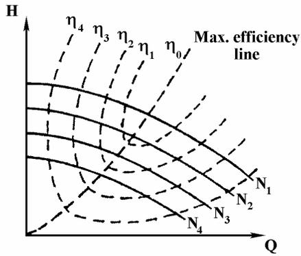
Fig. 4.8 Iso-efficiency curves
