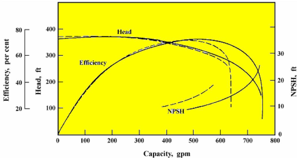
**Fig. 28 Effect of suction nozzle on NPSH requirements. 3-in. pump, 3500 rpm.**
