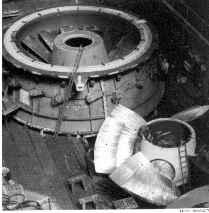
**Fig. 5.31** Workshop assembly of complete guide vane apparatus (two-part guide vane casing, 18 adjustable guide vanes in closed position) and of the runner
