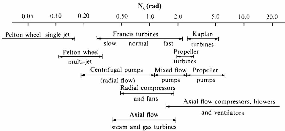
Fig. 2.7 Approximate specific speed and turbomachine type
