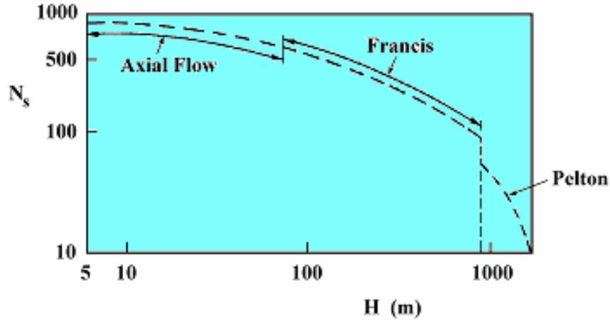
Fig. 5.21 Turbine classification according to specific speed and head
