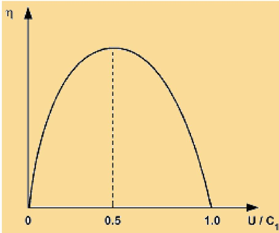
Fig. 5.3 Pelton wheel efficiency versus velocity ratio
