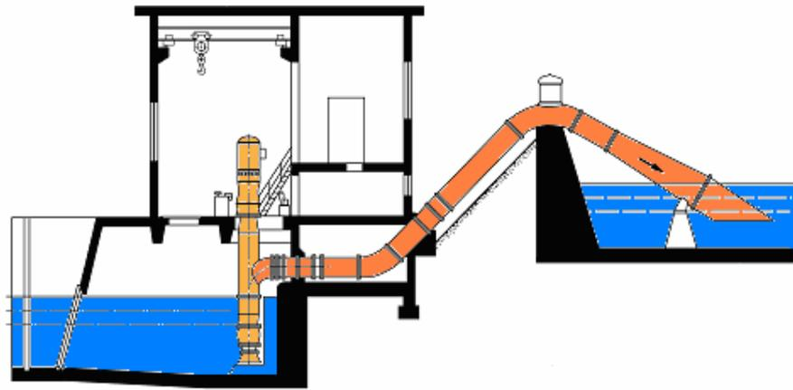
Fig. 4.48 Irrigation system using axial pumps (Courtesy of Sulzer Brothers)
