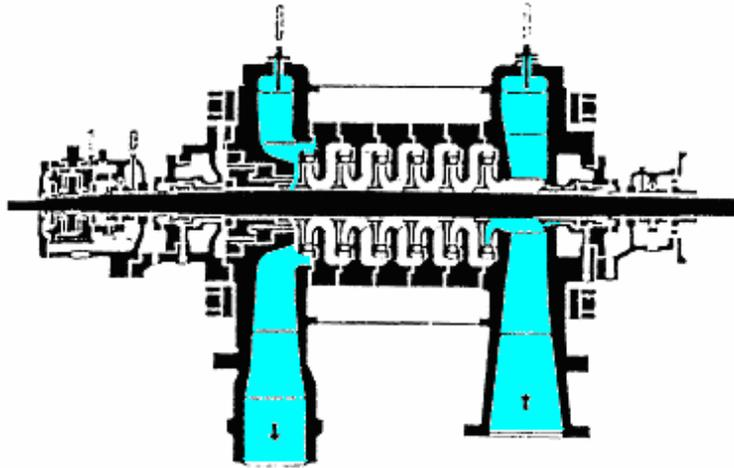
**Fig. 4.50 Multistage boiler feed pump (Courtesy of Sulzer Brothers)**
