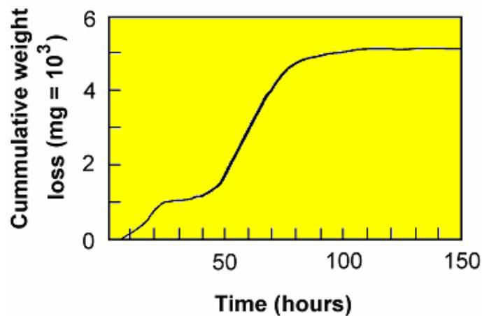
**Fig. 6 Cumulative weight loss versus the pump running time**
