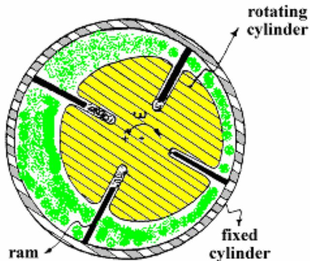
**Fig. 8.7 Radial cylinder rotary pump**
