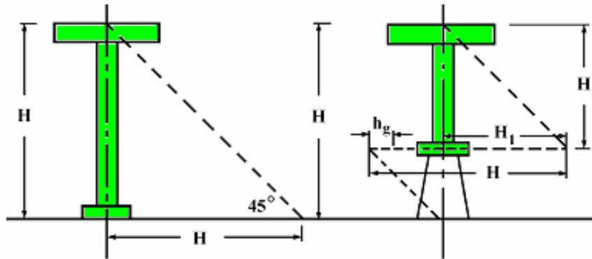
Fig. 5.17 Draft tube function
