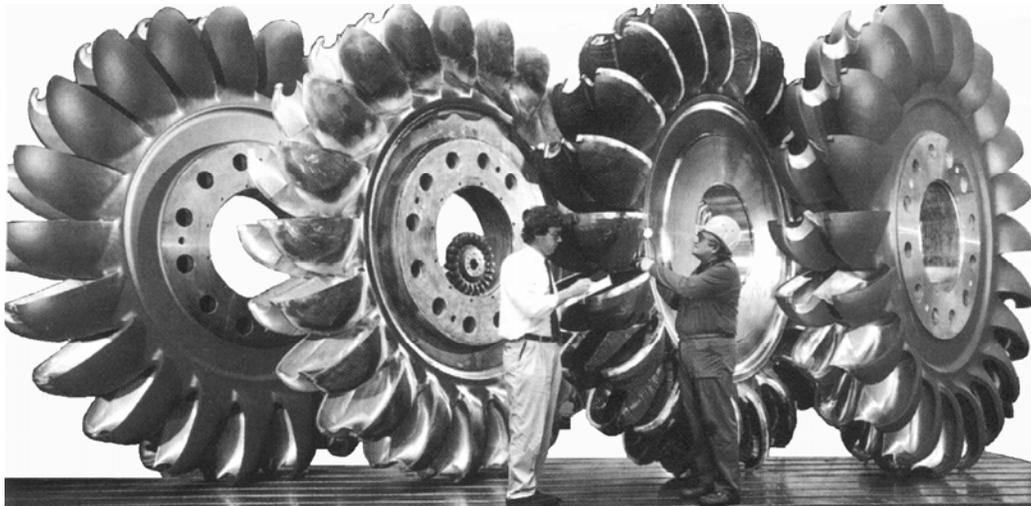
**Fig. 5.47** Four 260 MW Pelton turbine runners under a head of 1140 m with the model runner inside one of them
