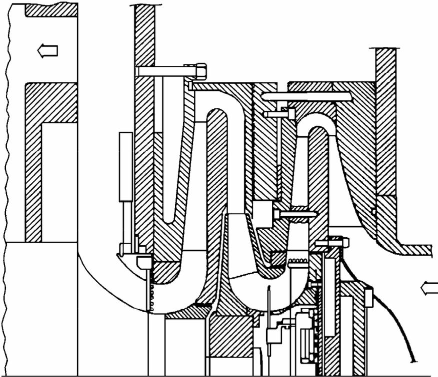
**Fig. 7.13** Sectional view in a centrifugal compressor showing one stage for test purposes (courtesy Nuovo Pignone)
