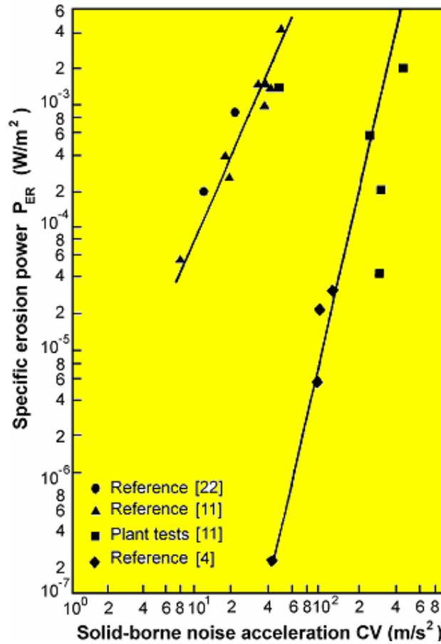
Fig. 20 Specific erosion power as a function of the solid-borne noise
