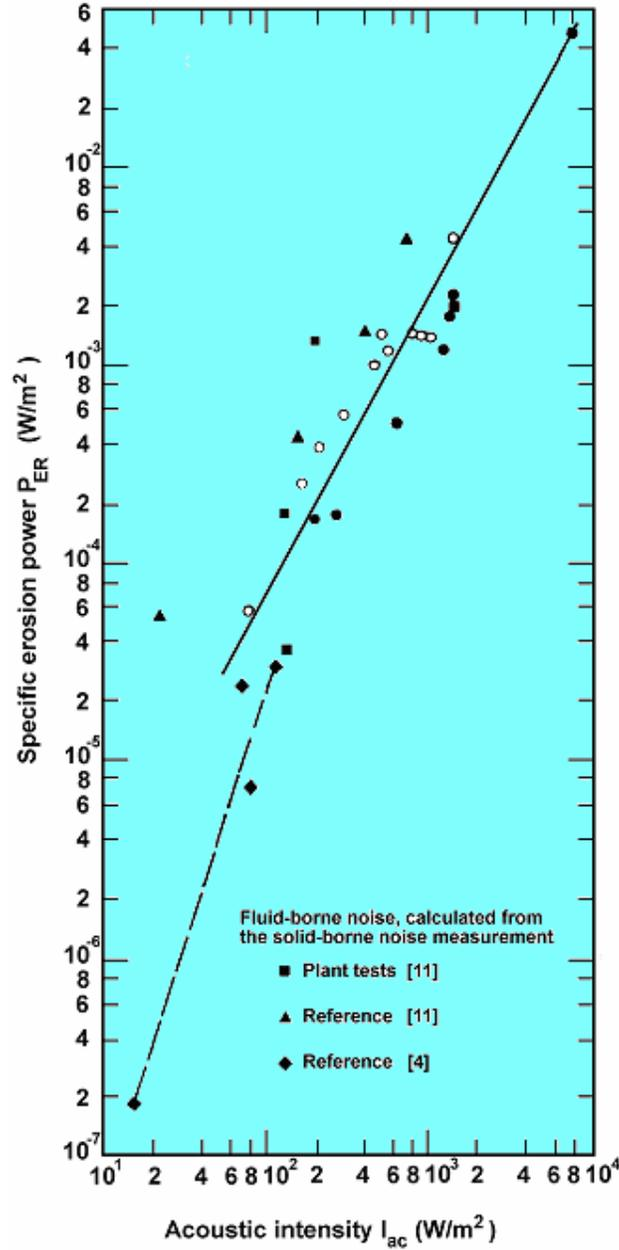
Fig. 22 Specific erosion power as a function of the fluid-borne noise
