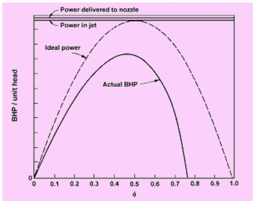
Fig. 5.7 Relation between power and speed at constant head
