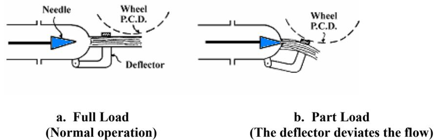
**Fig. 5.5 Speed and power regulation**
