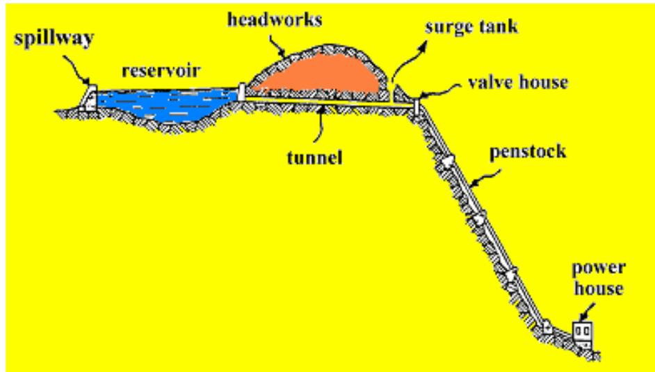
Fig. 5.26 Pelton wheel installation
