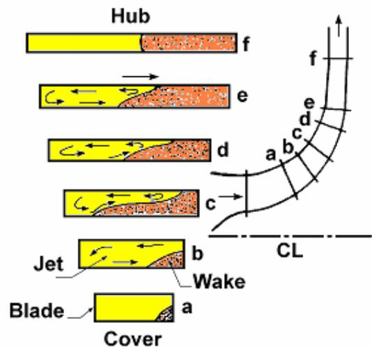
Fig. 2 (b) Development of the wake, secondary flow pattern (obtained by Dean, Jr.)
