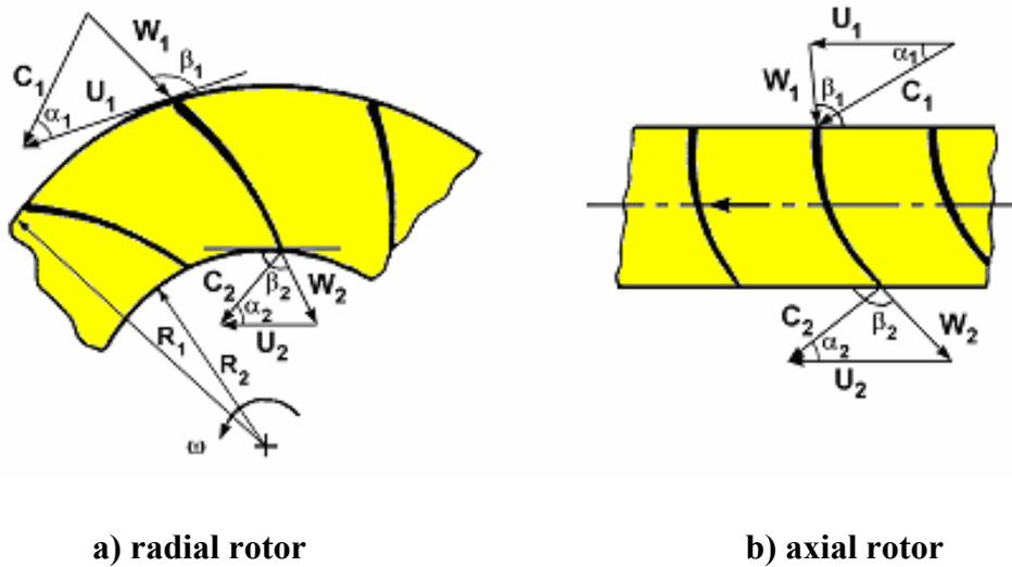
**Fig. 1.5 Inlet and exit velocity triangles**
