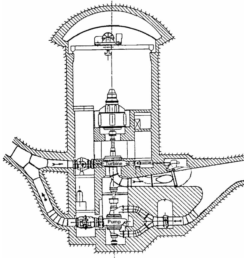
**Fig. 5.42** Section through the 51 m high cavern of the pumped-storage power station at Villa Gargnano (Italy). The intake sections of the pumps and the outlet sections of the turbines are connected to the Lake of Garda. The delivery pipes of the individual pump are combined with the pressure pipe of the turbine into single pipeline after the closing devices. The schedule provides for 3000 hours of running time. (Courtesy of Escher Wyss)
