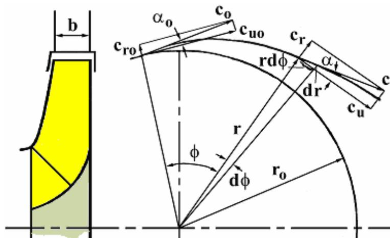
**Fig. 8 Spiral space with parallel side walls**
