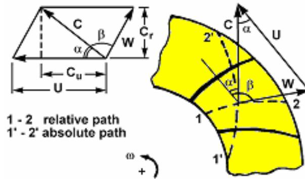
Fig. 1.2 Velocity triangle
