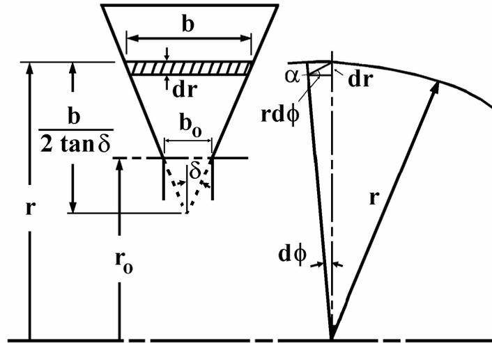
**Fig. 9 Tapering side wall diffuser**
