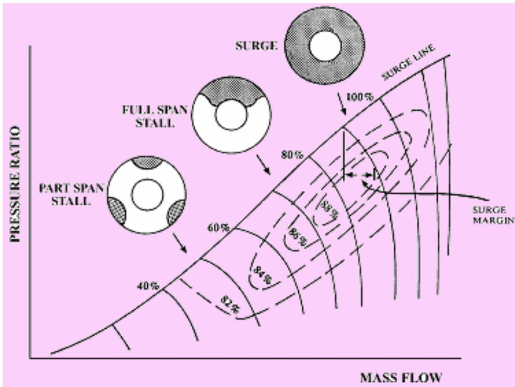
**Fig. 7.6 Performance curve for centrifugal compressor. Solid lines are characteristics at various speeds; dotted lines are corresponding efficiencies**
