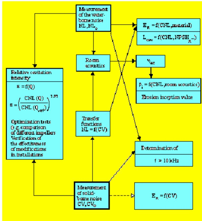
Fig. 23 Diagnosis possibilities available using fluid-borne and solid-borne noise
