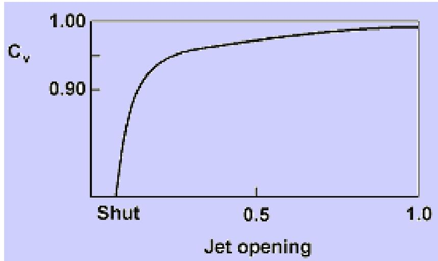
Fig. 5.4 Variation of  $C_v$  with jet opening
