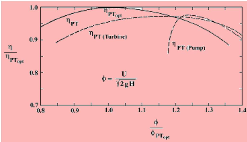
**Fig. 5.40** Relative efficiency as a function of relative pressure coefficient. In the operating range, the turbine and the pump efficiencies are at approximately equally high levels. The optimum turbine efficiency of the system is however lower than that of a conventional Francis turbine (Courtesy of Escher Wyss)
