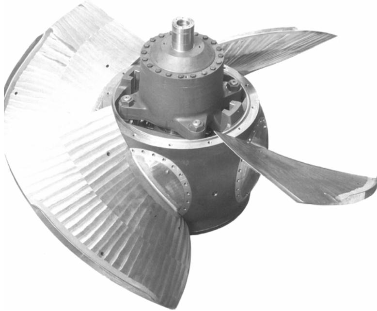
**Fig. 5.48 Kaplan runner for a bulb turbine (diameter 3.8 m, output 11.3 MW, head 14 m)**
