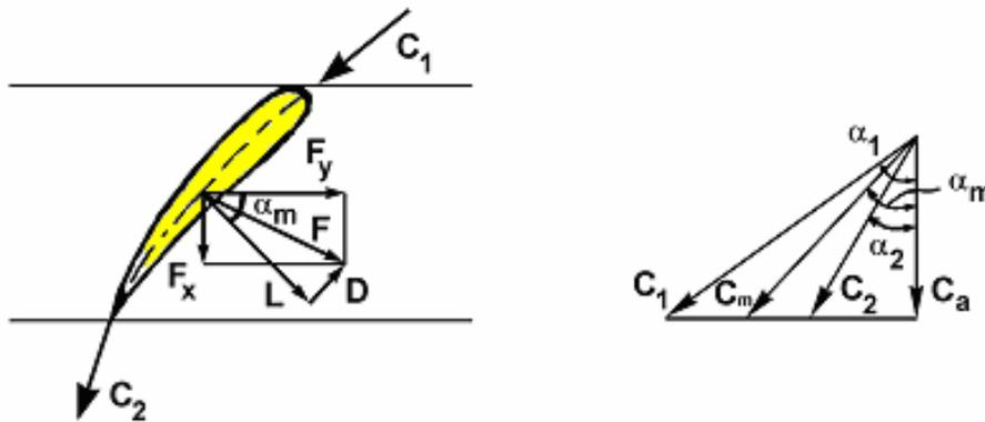
Fig. 3.3 Lift and Drag on cascade blade
