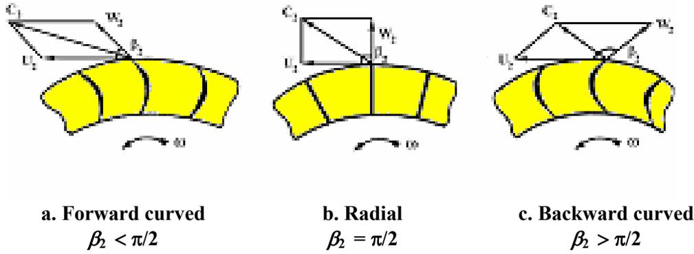
Fig. 4.3 Impeller exit angles
