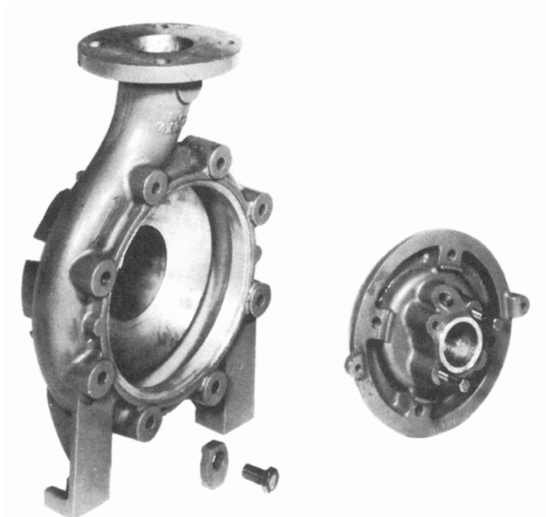
**Fig. 4.55 An offset-volute design of casing (left) and cover (right). The casing is designed for top centerline discharge, self-venting, and back pull-out**
