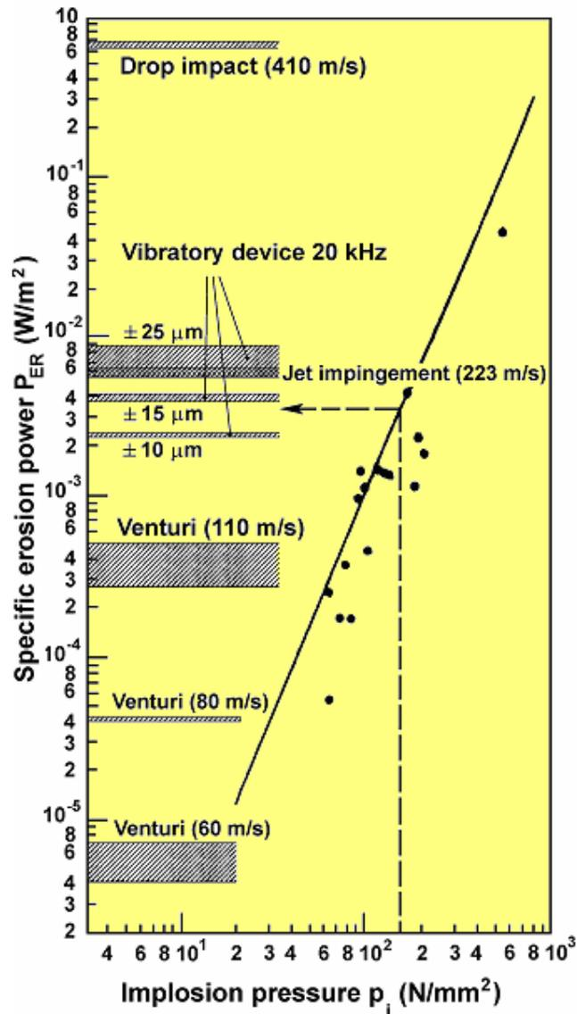
Fig. 18 Specific erosion power as a function of implosion pressure
