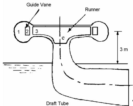
$$H_o = \frac{P_1}{\gamma} + \frac{C_1^2}{2g} + Z - \text{Losses}$$
