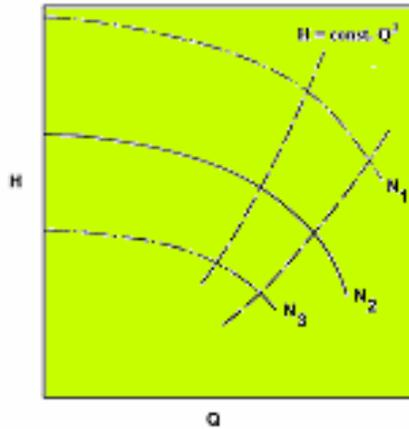
Fig 2.5 Head-capacity curve for a pump at different speeds
