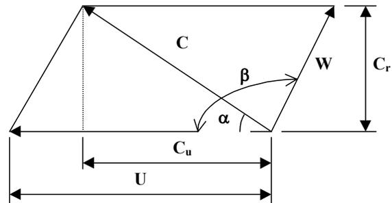
$C_r$  : the radial component of the absolute velocity
