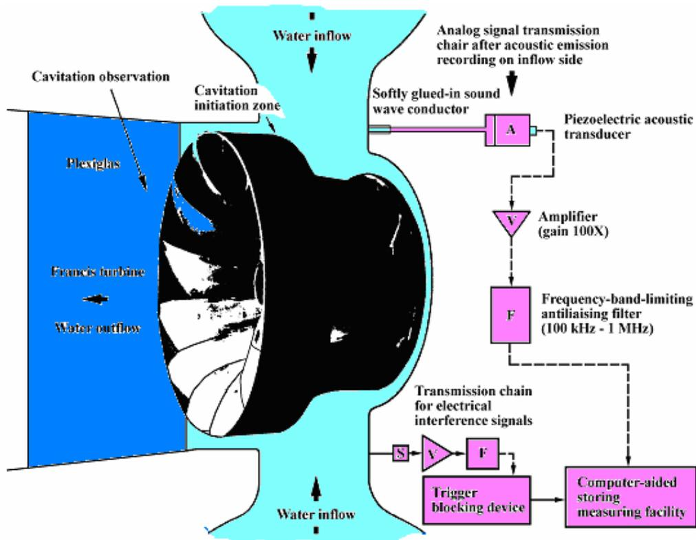
Fig. 27 AEA facility for cavitation investigation
