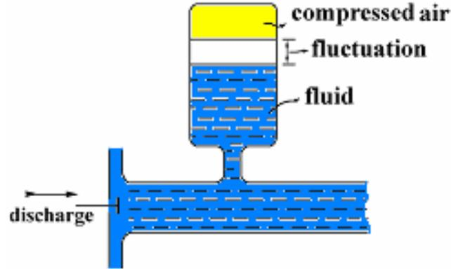
**Fig. 8.3 Air vessel**
