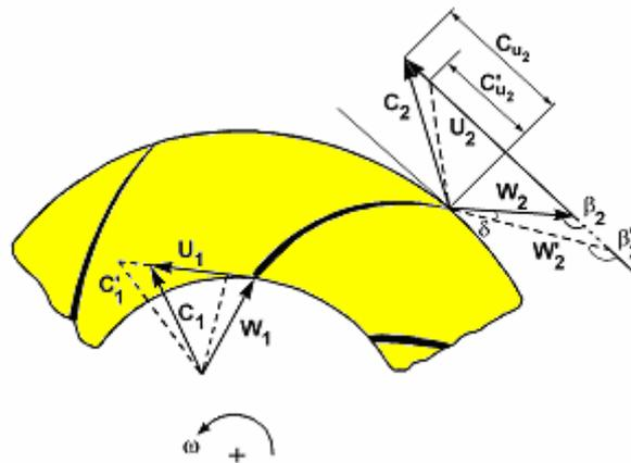
**Fig. 1.11 The velocity triangles after the modern theory**
