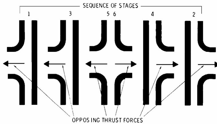
**a.2 Natural balancing achievement in a six-stage centrifugal pump, four impellers back-to-back and one double suction**
