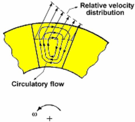
**Fig. 1.10 The flow pattern inside the impeller**
