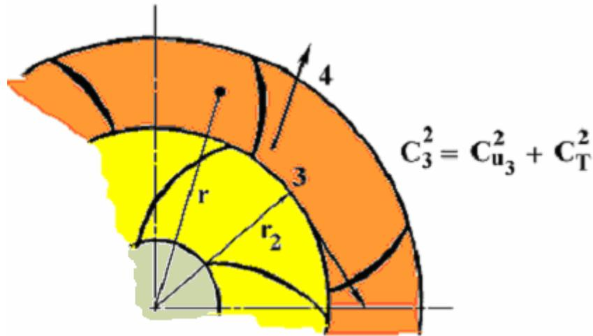
**Fig. 6 Vaned diffuser**
