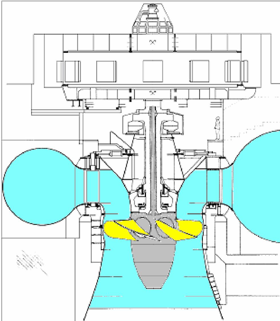
**Fig. 5.30 Turbine unit supported on three bearings.
