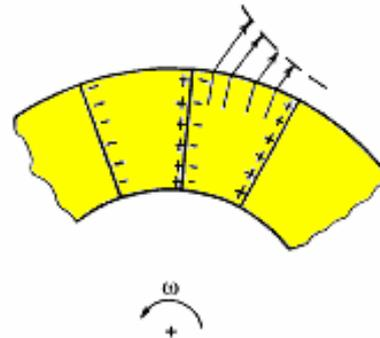
**Fig. 1.7 Exit flow shape in radial blades**
