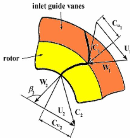
Fig. 5.14 Velocity triangles (inward turbine)
