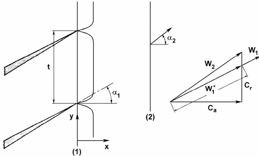
**Fig. 3 Boundary layer effects at the exit of a cascade**
