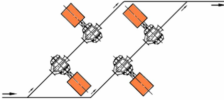
**a. Two standard pumps in series (each pump driven by its own individual motor)**
