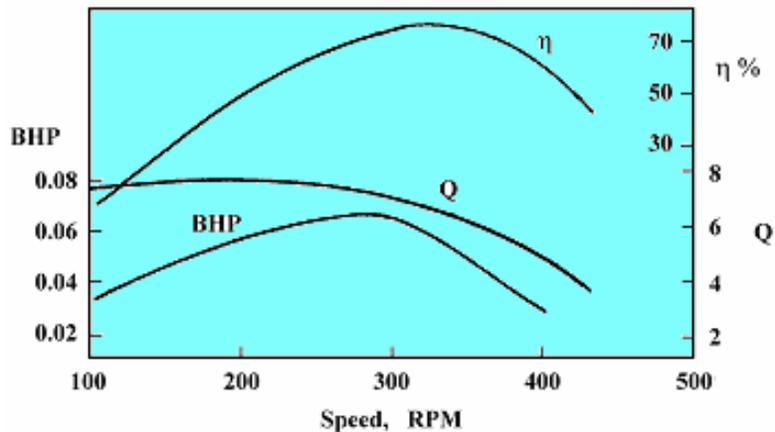
Fig. 5.23 Performance of Francis turbine running at 1 m head
