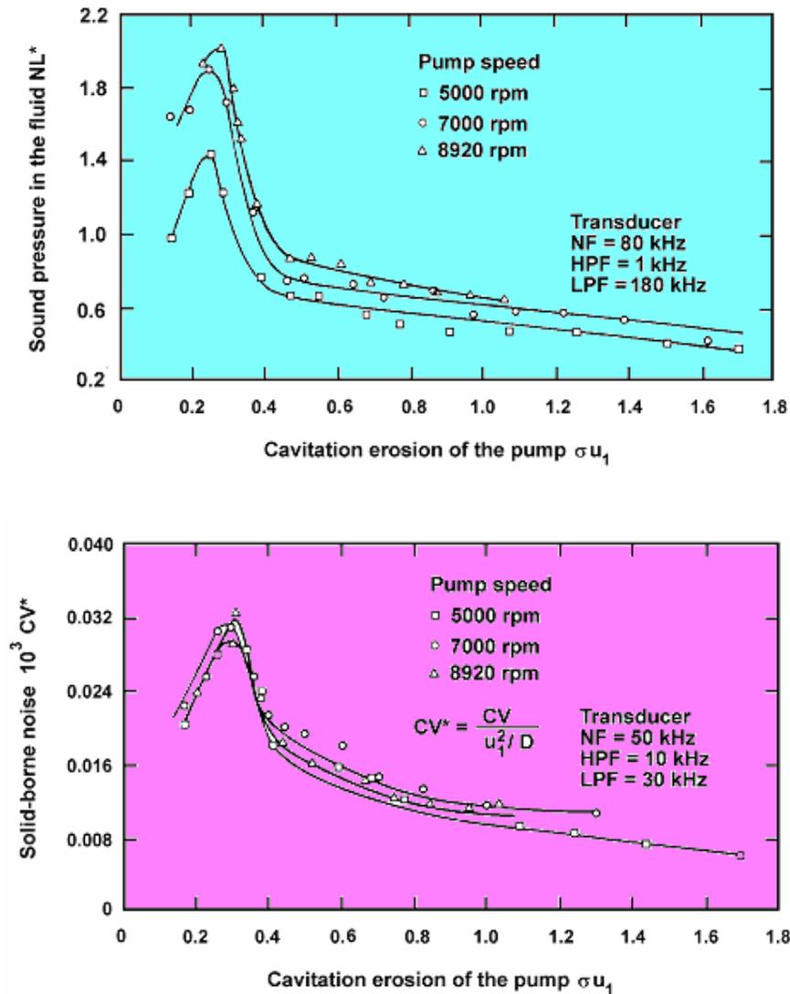
**Fig. 19 Fluid-borne and solid-borne noise – high-pressure pump**
