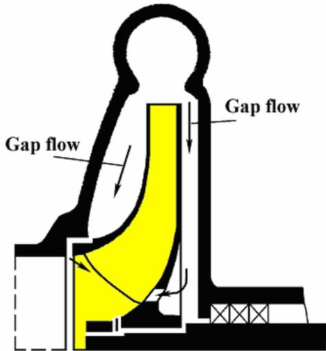
b. Single Stage Centrifugal Pump with Balance Holes
