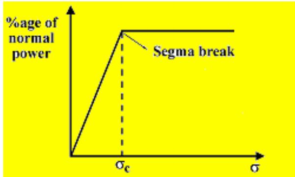
Fig. 5.19 Critical cavitation factor
