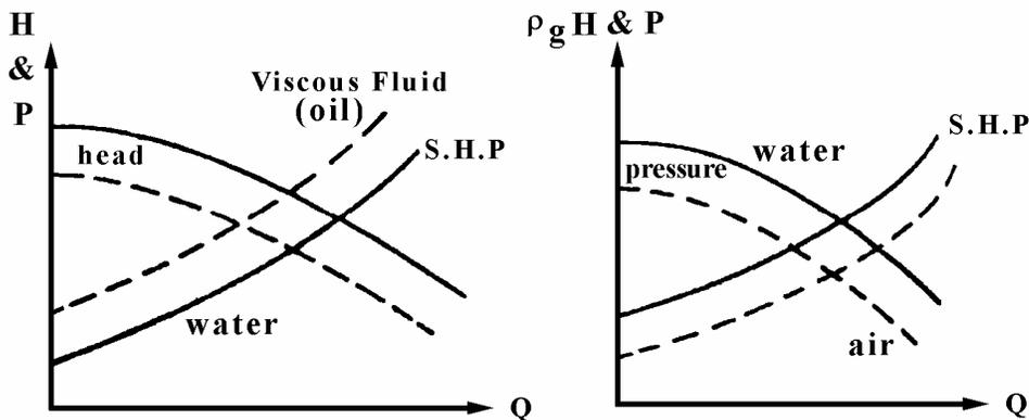
Fig. 4.10 Effect of viscosity and density on pump performance
