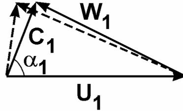
Fig. 1.15 Pre-rotation of the inlet velocity
