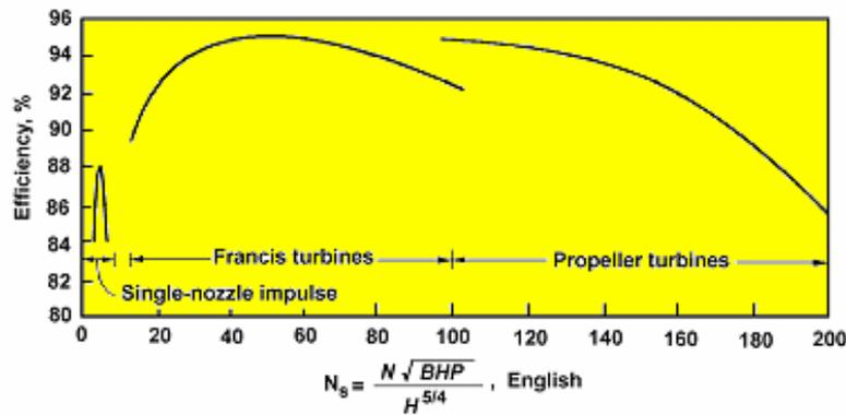
**Fig. 5.24 Maximum efficiency versus specific speed for different types of turbines**
