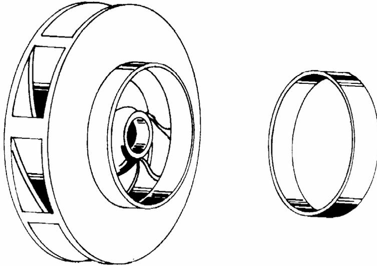
**Fig. 4.54 Enclosed-type double-inlet impeller and wearing ring. Some liquids require the impeller be made of special metals, such as chrome, monel, nickel, or a suitable alloy**
