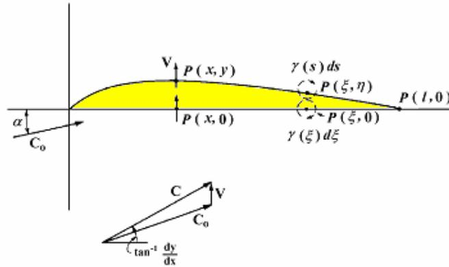
Fig. 3.15 An isolated thin airfoil
