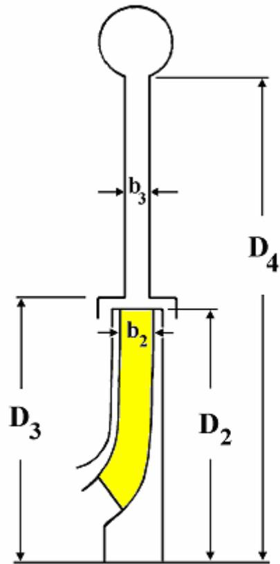
Fig. 4 Vaneless diffuser
