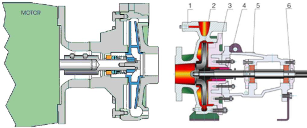
In cases where high-viscosity liquids (from about 120 mm<sup>2</sup>/s have to be pumped, a large spring or metal bellows must always be employed and the elbows must be relieved of torque transmission by suitable design. Auxiliary measures are often necessary with single seals too (Figure 4.13, Table 4.1).
