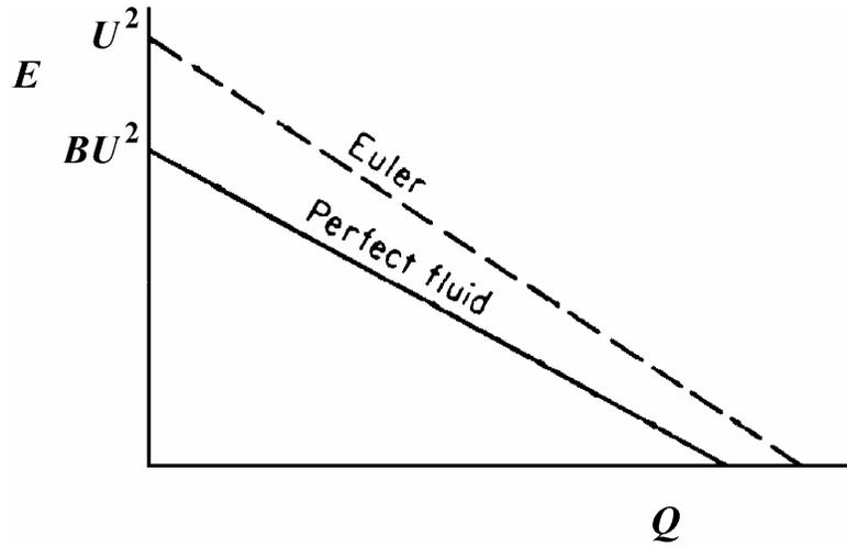
Fig. 3.13 Head-capacity curve for straight and radial cascades
