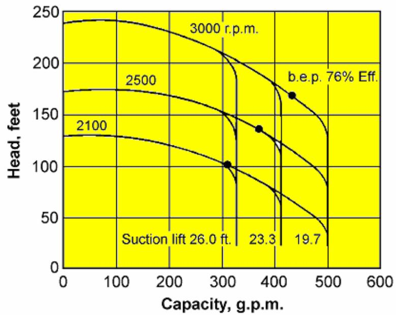
**Fig. 4 Effect of speed and suction lift on cavitation of a single-suction pump,  $N_s = 1000$**
