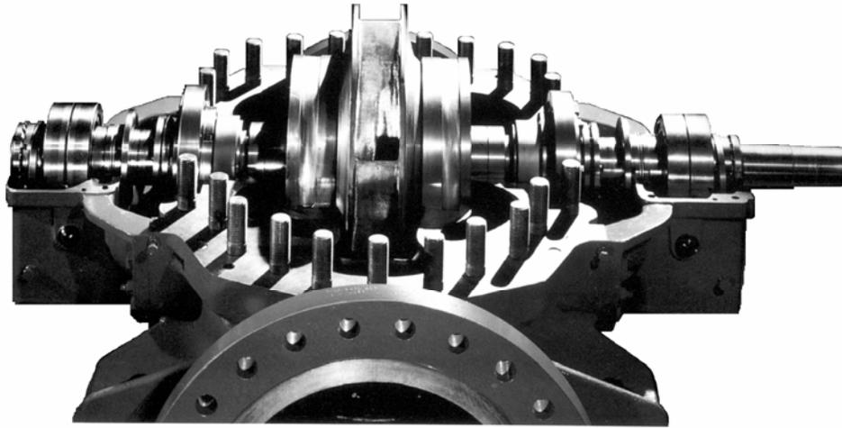
**Fig. 21 Sophisticated design and modern materials technology are particularly called for when cavitation cannot be completely avoided due to the given operating conditions**
