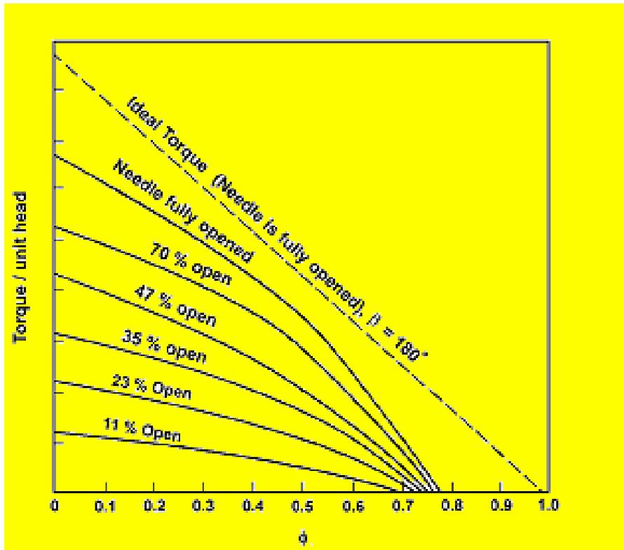
Fig. 5.6 Relation between torque and speed at constant head
