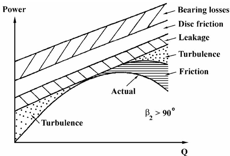
Fig. 4.6 Actual power-capacity curve
