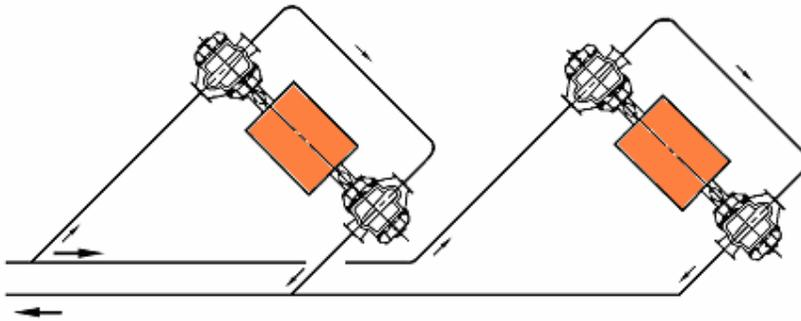
**b. Two standard pumps in series (each two pumps have one motor in common)**
