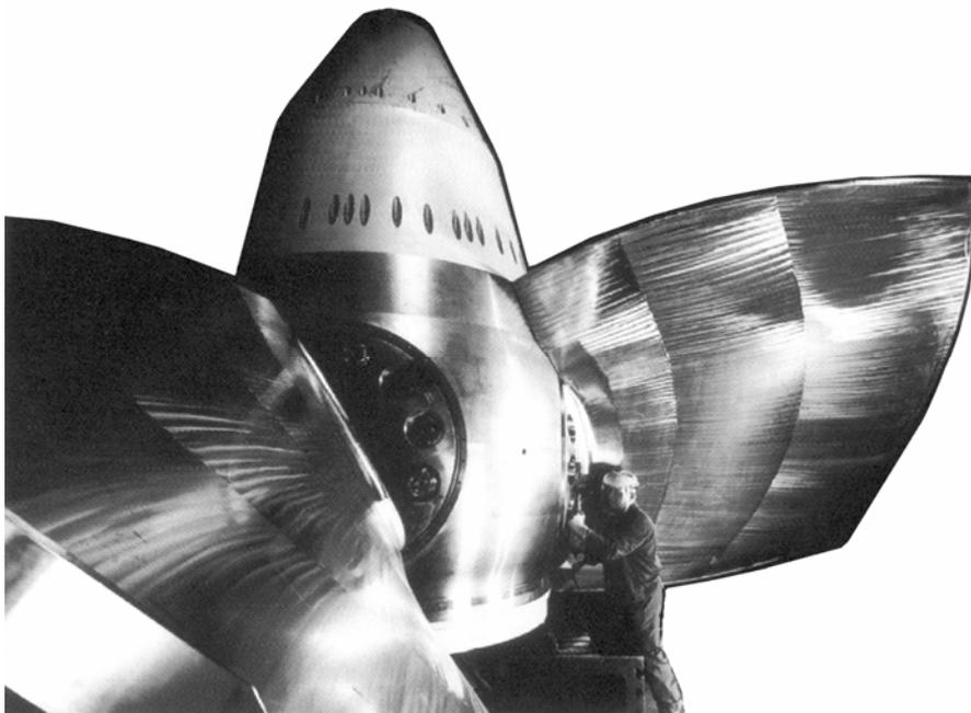
**Fig. 5.49 The Freudenau Kaplan bulb-turbine runners have a diameter of 7500 mm**
