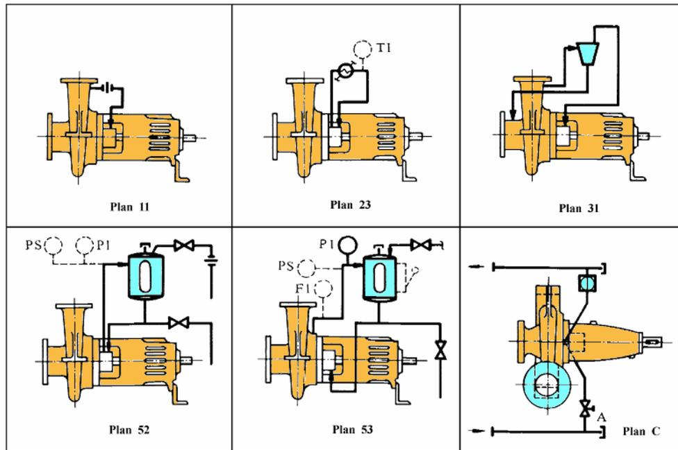
Fig. 4.13 Pipe work for auxiliary circuits to mechanical seals
