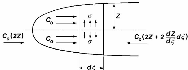
**Fig. 3.16 Allowance for profile thickness**
