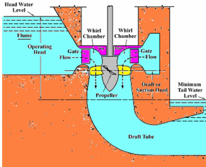
**Fig. 5.33 Axial turbine installation**
