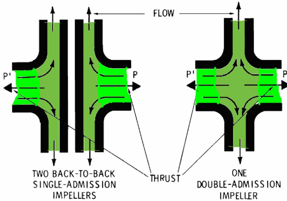
**a.1 Natural balancing achievement in single-stage pumps by means of two-back-to-back single-admission types of impellers (left) and one double-admission type of impeller (right)**
