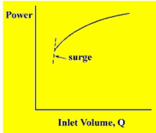
Fig. 7.5 Typical power-capacity curve for a centrifugal compressor
