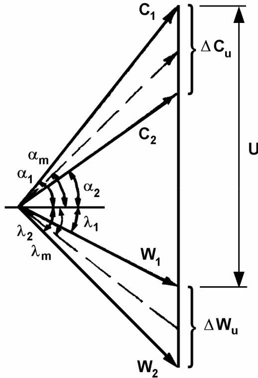
Fig. 3.4 Velocity triangle
