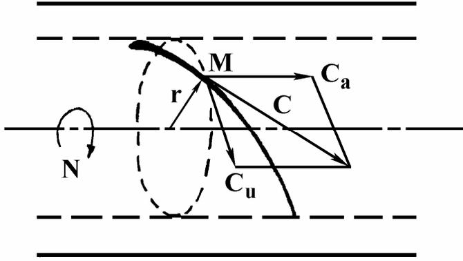
**Fig. 4.25 The trajectory of fluid particles could be co-axial cylinder**
