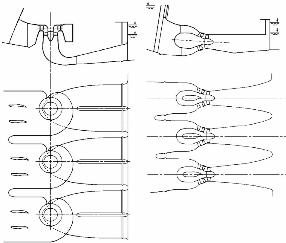
**Fig. 5.44 Comparison of amounts of space required by conventionally arranged Kaplan turbines (left) and tubular turbines with the same output (right). Less excavation work is required with tubular turbines, and the powerhouse can be made much lower and shorter, in view of the smaller distances between centres. The saving in volume of building space is therefore considerable**
