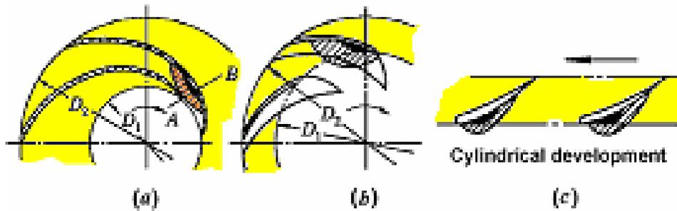
**Fig. 5 (a) Low pressure zones on back side of impeller vanes:**
