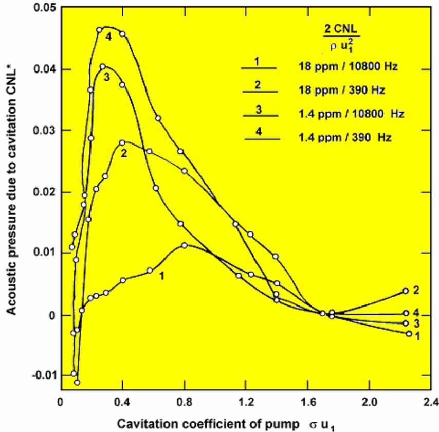
**Fig. 16 Influence of the air content and of the frequency range on the cavitation noise (high-pass filter set in each case at the given frequency)**
