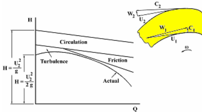
Fig. 4.5 Actual head-capacity curve
