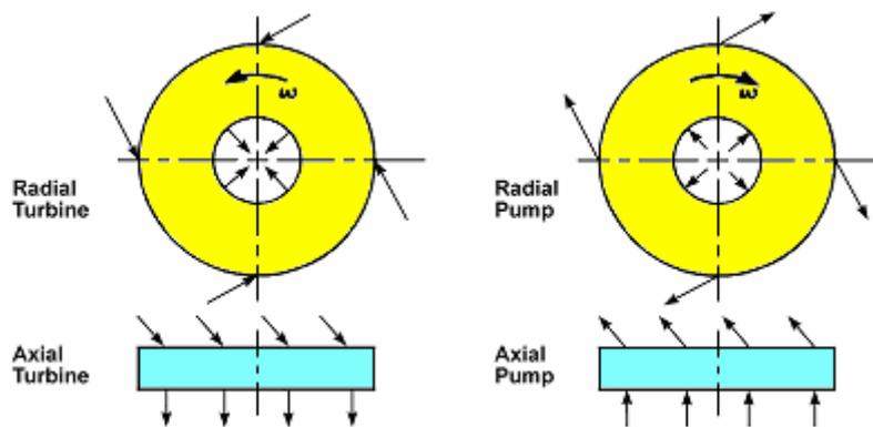
Fig. 1.1 Flow direction in turbines and pumps
