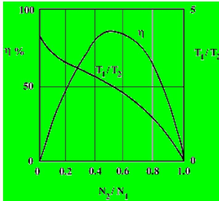
Fig. 5.39 Torque converter performance
