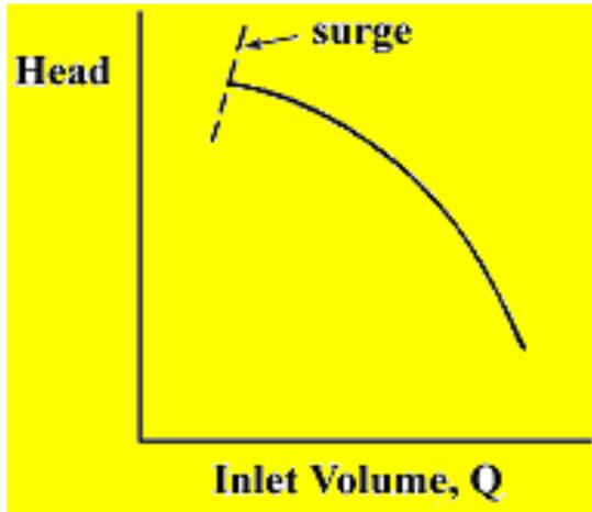
Fig. 7.4 Typical H-Q curve for a centrifugal compressor
