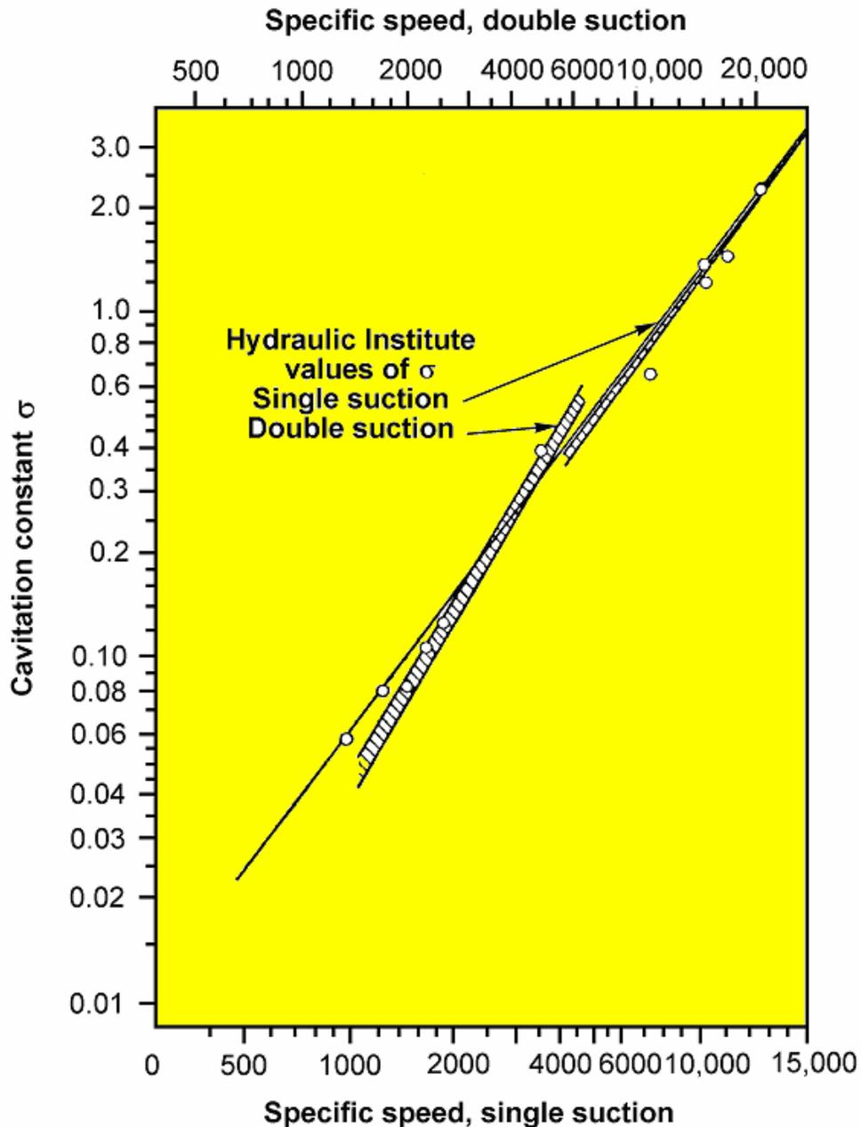
Fig. 14 Cavitation constant  $\sigma$  versus specific speed for best efficiency points
