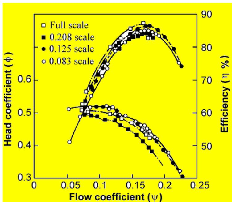
Fig. 2.4 Non-dimensional presentation of model and full size performance for the Eggborough pump (adapted from Nixon and Cairney, 1972)
