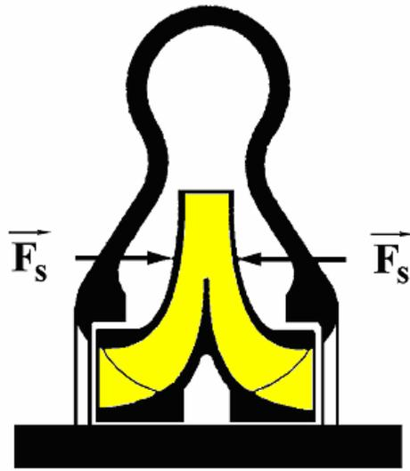
a.3. Double Suction Impeller Arrangement
