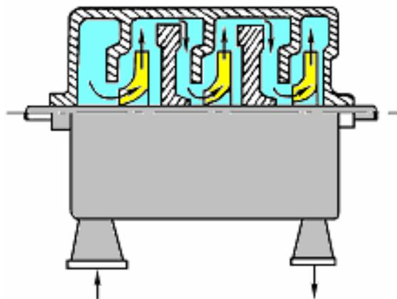
Fig. 7.2 Three-stages turbo-compressor
