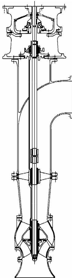
**Fig. 4.51 Vertical axial pump (Courtesy of Sulzer Brothers)**
