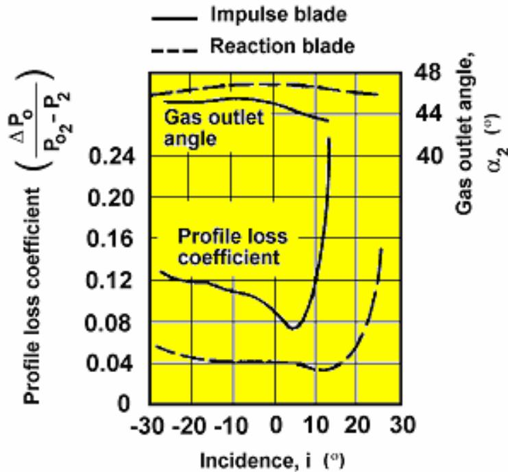
Fig. 3.9 Variation in profile loss with incidence for typical turbine blades after Ainley (adapted from Dixon)
