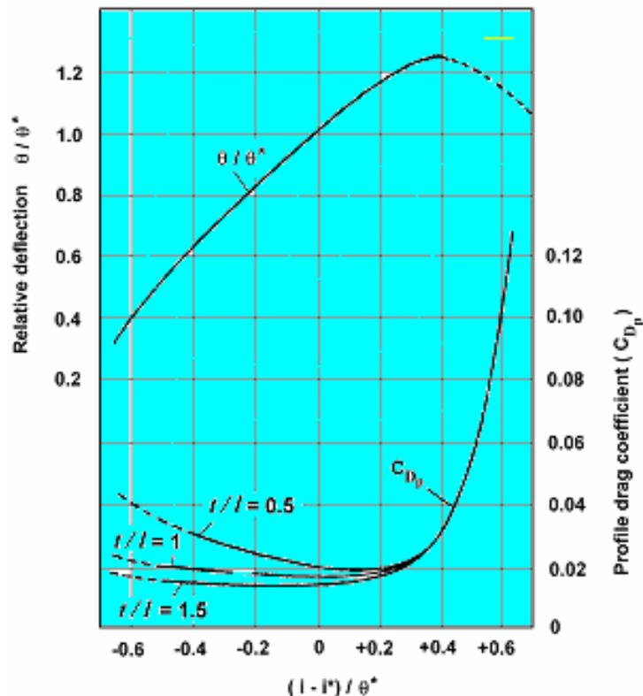
Fig. 3.8 The off-design performance of a compressor cascade (after Howell)
