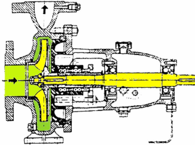
Fig. 4.49 A section in a radial centrifugal pump (Courtesy of Sulzer Brothers)
