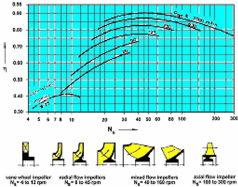
Fig. 2.6 Approximate relative impeller shapes and good average efficiencies obtained for commercial pump as a function of specific speed,
