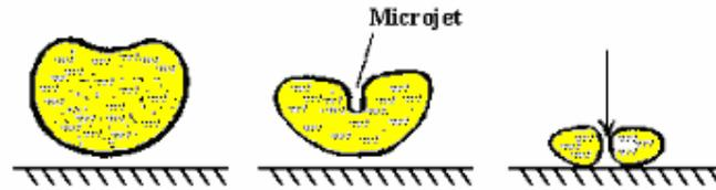
Fig. 7 (b) Schematic representation of successive stages of nonsymmetrical cavity collapse with microjet impingement against a metallic surface
