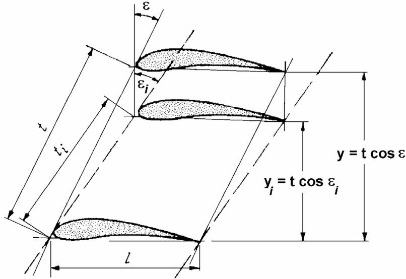
**Fig. 3.10 Geometry of the real and the equivalent cascade, *i* denotes parameters referring to equivalent cascade in incompressible flow**
