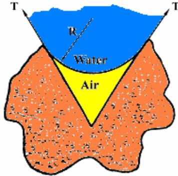
**Fig. 1 A condition whereby an air bubble can remain stable indefinitely, without solution on a hydrophobic particle possessing a concave surface (after Liebermann)**
