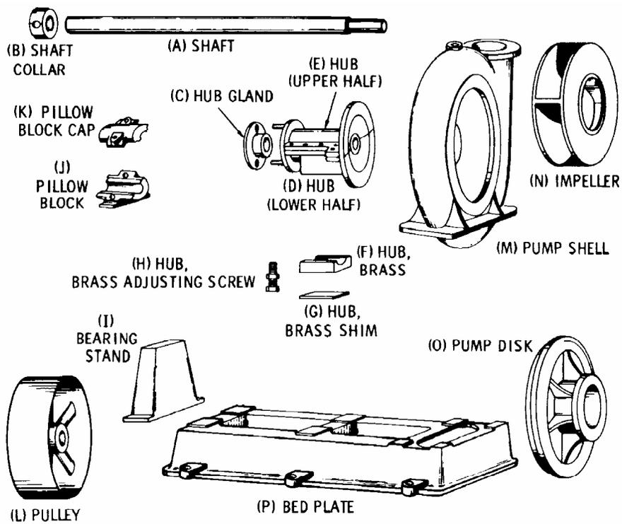
**Fig. 4.57 Disassembly view showing parts of a belt-driven single-stage centrifugal pump. The parts shown are: (A) shaft; (B) shaft collar; (C) hub gland; (D) hub (lower half); (E) hub (upper half); (F) hub, brass; (G) hub, brass shim; (H) hub, brass adjusting screw; (I) bearing stand; (J) pillow block; (K) pillow-block cap; (L) pulley; (M) pump shell; (N) impeller; (O) pump disk; (P) bed plate**
