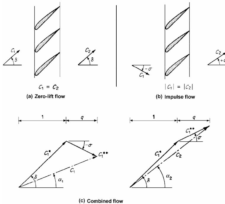
**Fig. 3.11 Zero-lift and impulse flow angles**
