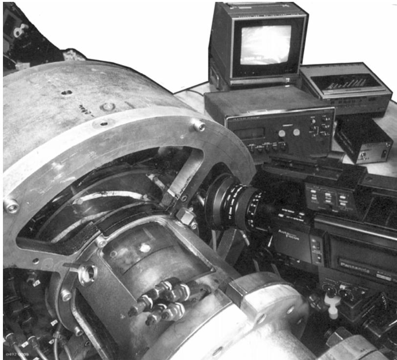
**Fig. 17** Bubble field observations using the stroboscope require expensive modifications to the pumps. Cavitation noise measurements carried out at the same time provide clarifying information for use in the interpretation of fluid-borne and solid-borne noise
