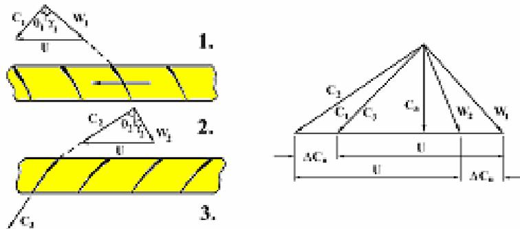
Fig. 4.23 Pressure and flow coefficients
