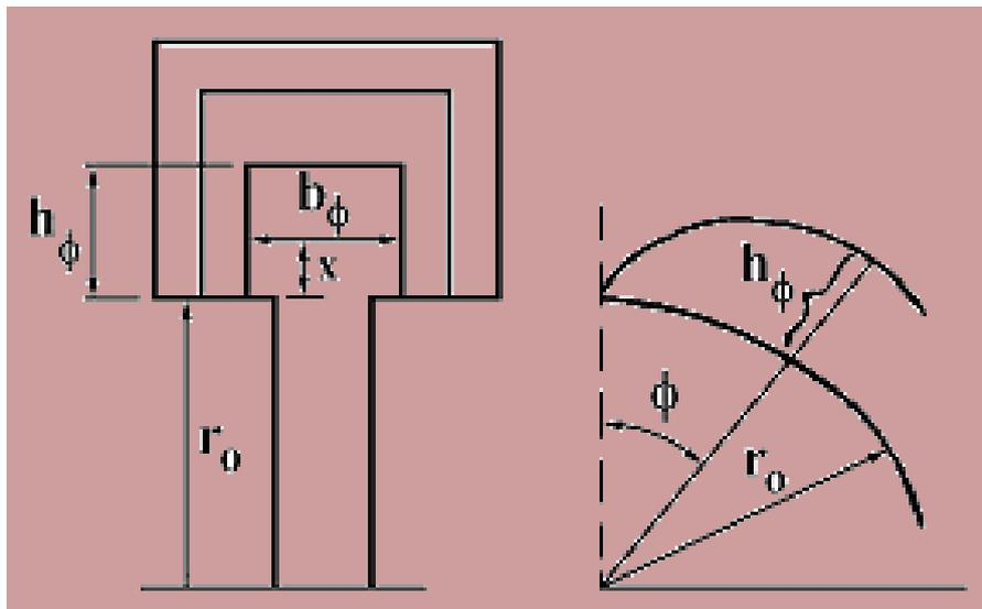
**Fig. 10 Rectangular cross section diffuser**
