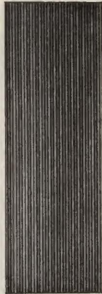
FIG. 29.6 Fresnel's biprism interference bands (magnified).
