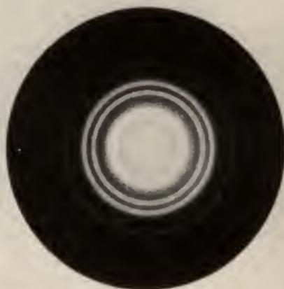
(ii) Electron diffraction rings produced by a thin gold film.
