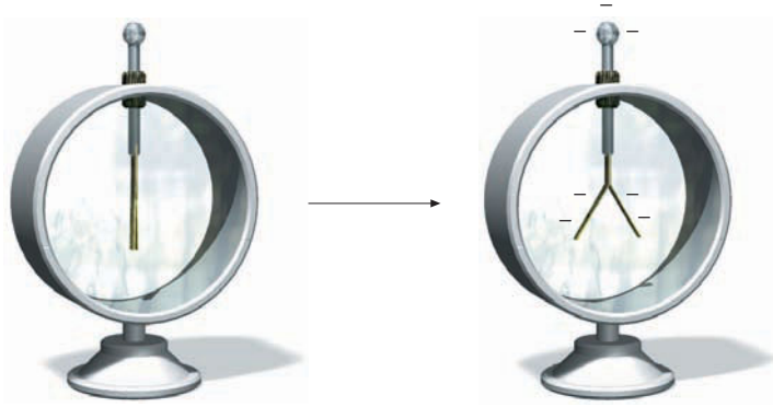
FIGURE 21-2 An electrostatic demonstrator. Two gold leaves are attached to a conducting post that has a conducting ball on top. The ball, post, and leaves are insulated from the container. When uncharged, the leaves hang together vertically. When the ball is touched by a negatively charged plastic rod, some of the negative charge from the rod is transferred to the ball and moves to the gold leaves, which then spread apart because of electrical repulsion between their negative charges. (Touching the ball with a positively charged glass rod would also cause the leaves to spread apart. In this case, the positively charged glass rod would remove electrons from the metal ball, leaving a net positive charge on the ball, rod, and leaves.)
