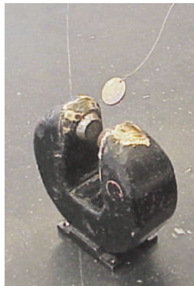
A Canadian quarter that is attracted by a magnet. Canadian coins often contain significant amounts of nickel, which is ferromagnetic. (Photo by Gene Mosca.)
