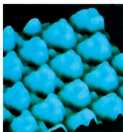
Benzene molecules of the order of 10^{-10} m in diameter as seen in a scanning electron microscope. (IBM Research, Almaden Research Center.)
