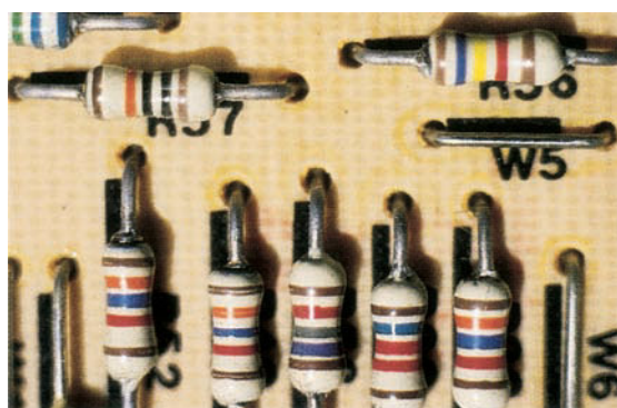
Color-coded carbon resistors on a circuit board. (© Chris Rogers/The Stock Market.)
