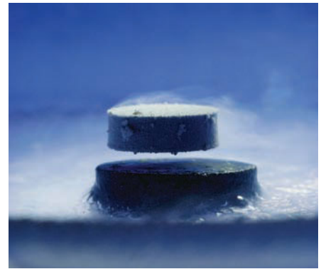
The disk is a superconductor. The magnetic levitation results from the repulsion between the permanent magnet producing the applied field and the magnetic field produced by the currents induced in the superconductor. (© Palmer/Kane, Inc./CORBIS.)
