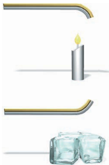
FIGURE 17-2 A bimetallic strip. When heated or cooled, the two metals expand or contract by different amounts, causing the strip to bend.
