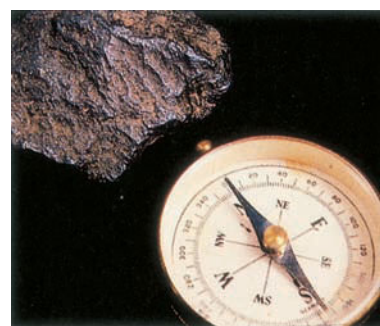
A chunk of magnetite (lodestone) attracts the needle of a compass. (© Paul Silverman/ Fundamental Photographs .)
