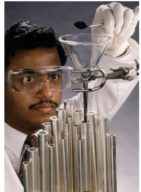
The researcher is filling tubes with high-temperature superconducting powder in order to make wire. (Courtesy of Department of Energy.)
