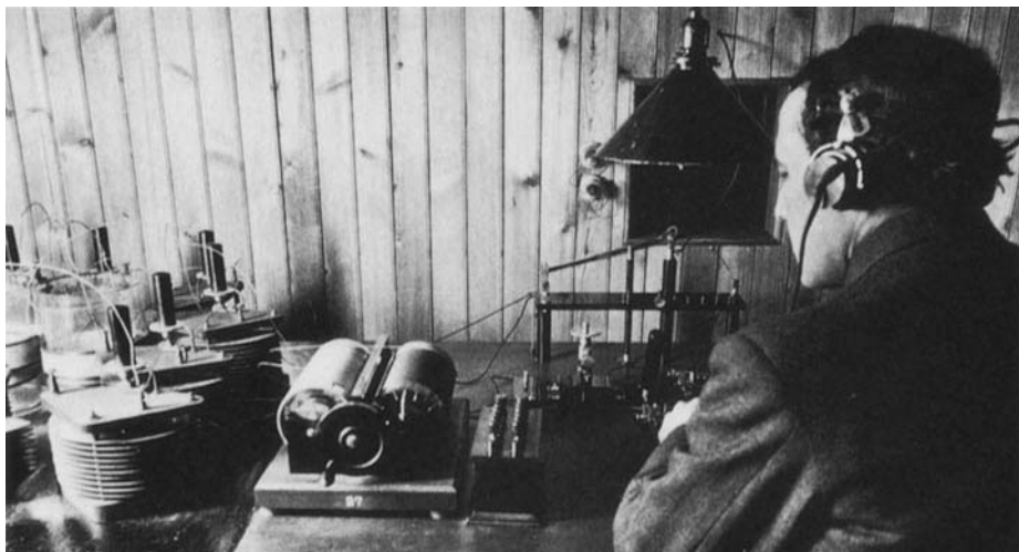
A shipboard radio, circa 1920. Exposed at the operator’s left are the inductance coils and capacitor plates of the tuning circuit. (© George H. Clark Radioana Collection-Archive Center, National Museum of American History.)
