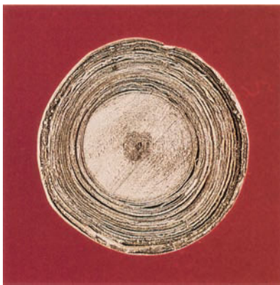
Cross section of a foil-wound capacitor. ( © Bruce Iverson. )
