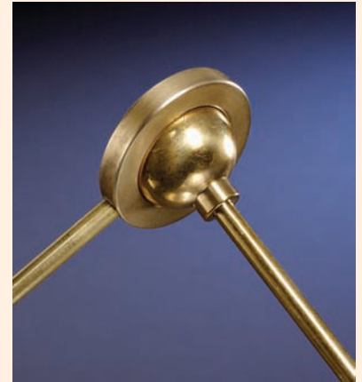
FIGURE 20-1 When the ball and ring are both at room temperature, the ball is too big to pass through the ring. The ring expands when heated, and when it is hot the ball, which remains at room temperature, is able to pass through the hole. (Richard Megna/Fundamental Photographs.)
