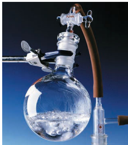
FIGURE 17-7 Water at its triple point. The spherical flask contains liquid water, ice, and water vapor in thermal equilibrium. (Richard Menga/Fundamental Photographs.)
