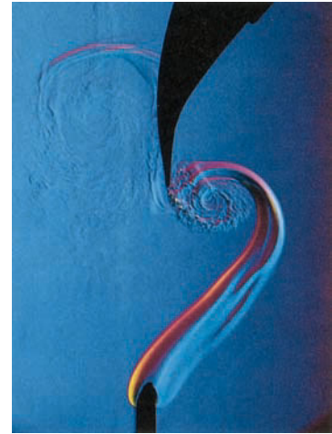
Smoke from a burning cigarette. At first the smoke rises in a regular stream, but the simple streamlined flow quickly becomes turbulent and the smoke begins to swirl irregularly. (Estate of Harold E. Edgerton.)
