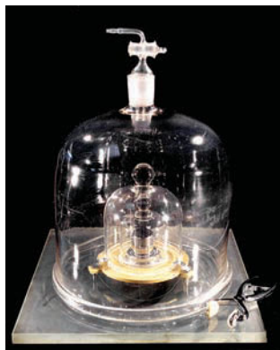
The standard body is the mass of a specific platinum-iridium alloy cylinder that is kept at the International Bureau of Weights and Measures in Sèvres, France. (© BIPM; www.bipm.org .)
