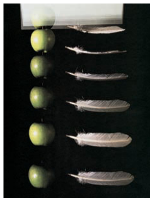
FIGURE 2-19 In a vacuum the apple and the feather, released simultaneously from rest, fall with identical motion. (James Sugar/Black Star.)
