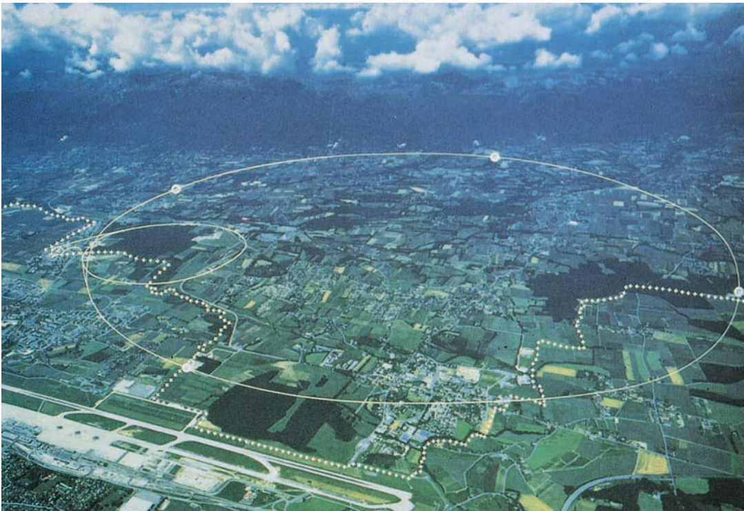
An aerial view of the European Laboratory for Particle Physics (CERN) just outside of Geneva, Switzerland. The large circle shows the Large Electron–Positron collider (LEP) tunnel, which is 27 km in circumference. The irregular dashed line is the border between France and Switzerland. (Richard Ehrlich.)
