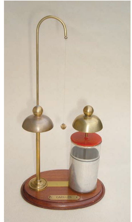
FIGURE 24-1 Leyden jar with bells. The bell on the pole through the stopper is connected to a conductor on the inside surface of the jar. The second bell is connected to the conductor on the outside surface of the jar. The system is energized by connecting a battery between the two bells for a short time. After the battery is removed the conducting ball swings from one bell to the other, transferring charge a little bit at a time. (Courtesy of Bernhard Thomas.)
