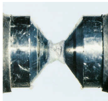
Liquid oxygen, which is paramagnetic, is attracted by the magnetic field of a permanent magnet. A net force is exerted on the magnetic dipoles because the magnetic field is not uniform. (J. F. Allen, St. Andrews University, Scotland.)
