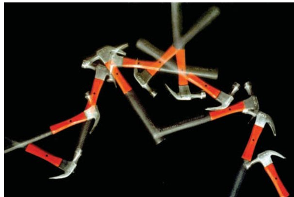
FIGURE 5-48 The center of mass (the black dot) of the hammer moves in a smooth parabolic path. (LorenWinters/Visual Unlimited.)
