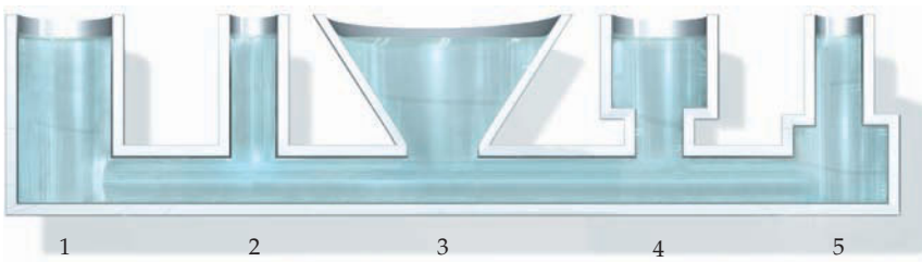
FIGURE 13-6 The hydrostatic paradox. The water level is the same regardless of the shape of the vessel. The weight of those portions of the water not above an opening is supported by the sides of the containers.
