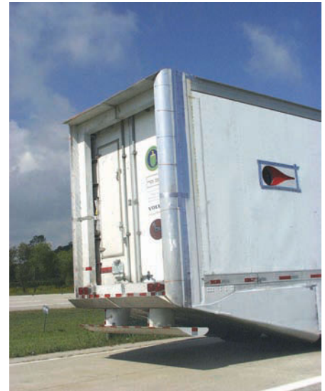
At highway speeds aerodynamic drag is reduced because of the jets of air along the back edge of the truck body of this prototype. (Courtesy of Georgia Institute of Technology.)
