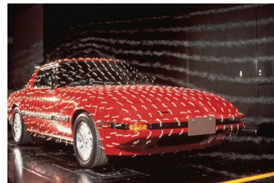
Streamlined body designs can greatly reduce the drag forces on moving objects such as automobiles or airplanes. (Takeski Takahara/Photo Researchers, Inc.)
