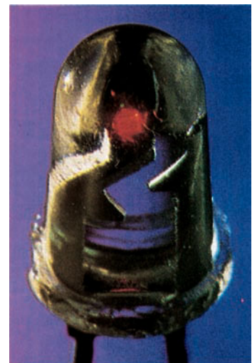
A light-emitting diode (LED). (© C. Falco/Photo Researchers.)
