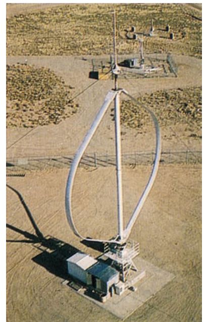
An experimental wind-powered electric generator at Sandia National Laboratory. The propeller is designed for optimum transfer of wind energy to mechanical energy. (Sandia National Laboratory.)
