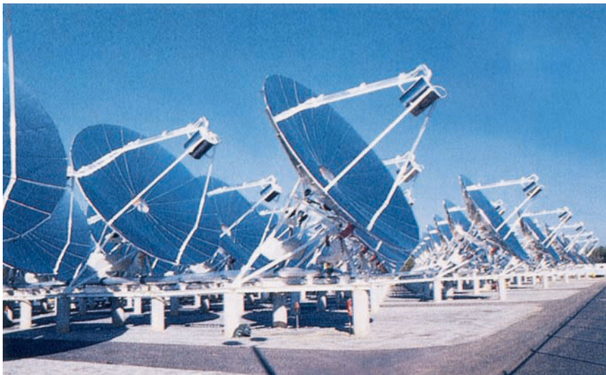
Solar energy is focused and collected individually for these heliostats, which are being tested at Sandia National Laboratory, to produce electricity. ( Sandia National Laboratory. )
