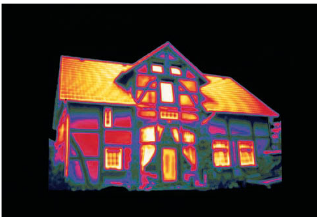
This thermogram of a house shows the heat being radiated to its surroundings. (Alfred Pasiaka/Photo Researchers, Inc.)
