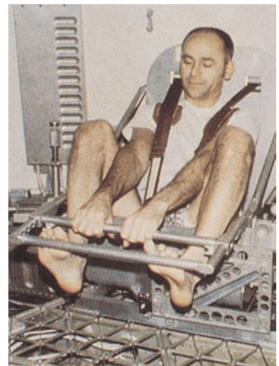
Astronaut Alan L. Bean measures his body mass during the second Skylab mission by sitting in a seat attached to a spring and oscillating back and forth. The total mass of the astronaut plus the seat is related to his frequency of vibration by Equation 14-12. (NASA.)
