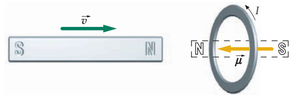
FIGURE 28-9 The magnetic moment of the loop \vec{\mu} (shown in outline as if it were a bar magnet) due to the induced current is such as to oppose the motion of the bar magnet. The bar magnet is moving toward the loop, so the induced magnetic moment repels the bar magnet.
