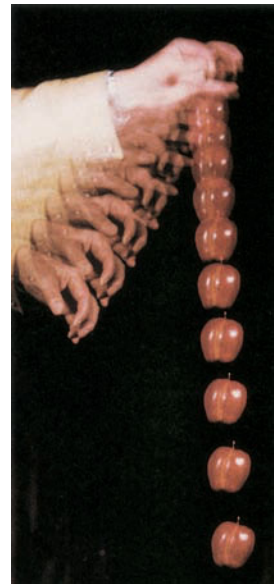
A falling apple captured by strobe photography at 60 flashes per second. The acceleration of the apple is indicated by the widening of the spaces between the images. (Estate of Harold E. Edgerton/Palm Press.)
