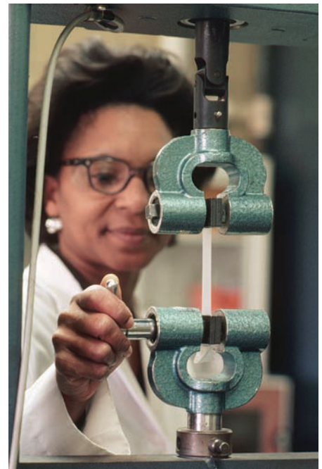
To measure the tensile strength, the rod is stretched until it breaks. (Vince Streato/CORBIS.)
