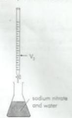
Prom the titration result, we can know the exact volume of nitric acid needed to react with 25.0 cm<sup>3</sup> of sodium hydroxide. Volume of nitric acid, V<sub>x</sub> = V<sub>2</sub> - V<sub>1</sub>
